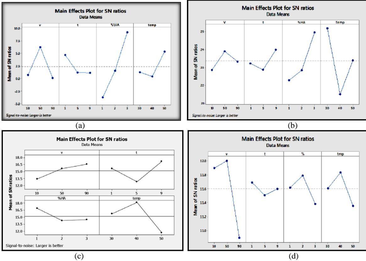
Figure 7: SNs ratio (a) %porosity, (b) thickness, (c)nanoroughness and (d) microughness.
