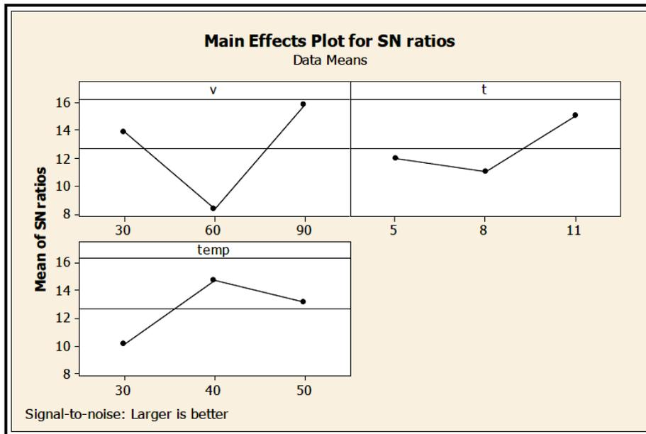
Figure 2: Mean of SNs response for chitosan thickness for different variables and levels
