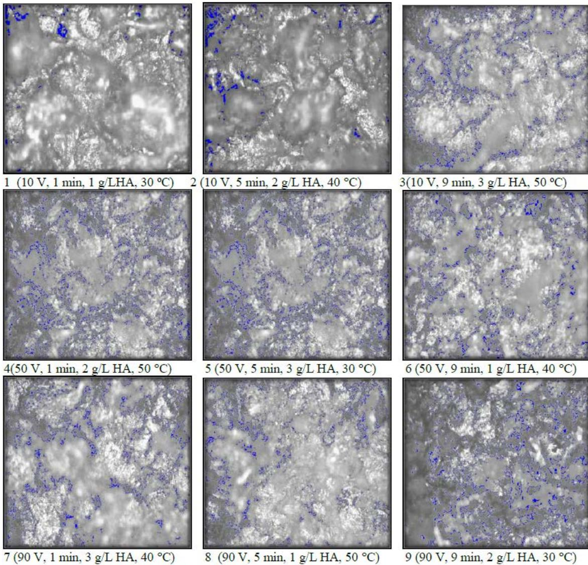
**Figure 4:** Optical images of porosity for HA coating (blue color refer to pores area).
