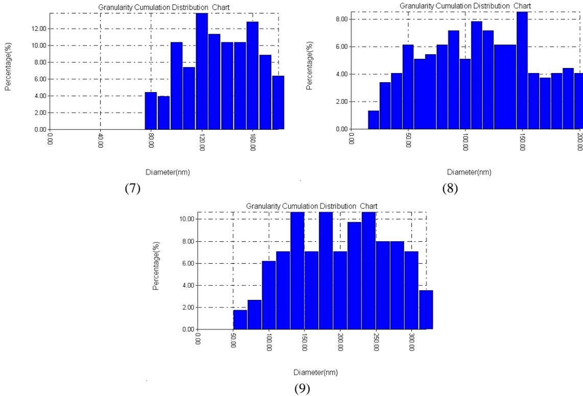
**Figure 6:** Charts of granularity accumulation for coating particles of HA coating layer for different samples.
