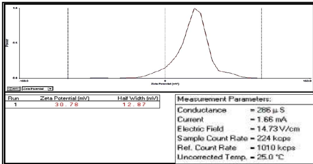
**Figure 1:** The value of zeta potential for chitosan solution at 90 V, 40°C and 11 min.
