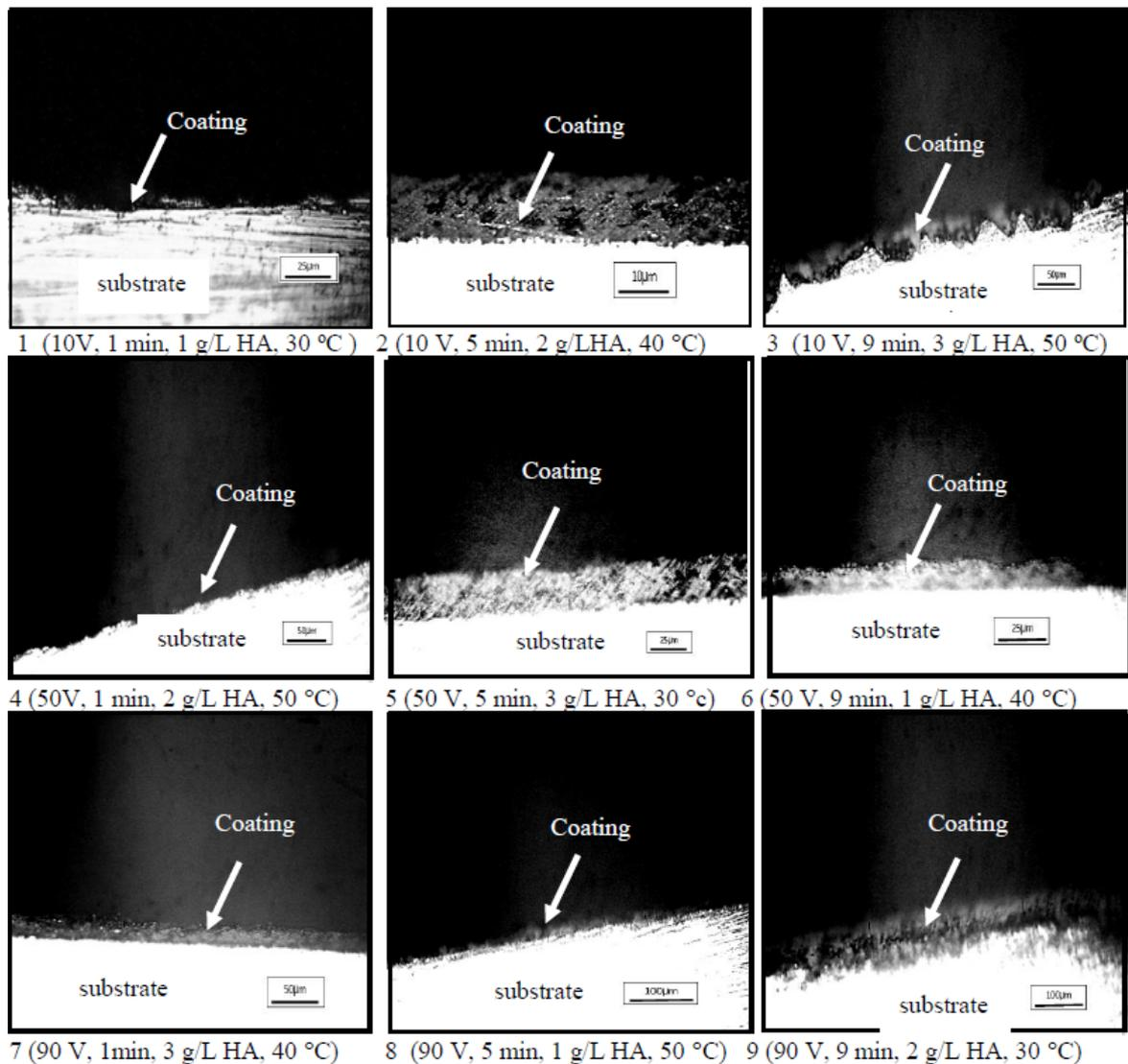
Figure 3: Optical microscopy images for samples of HA/chitosan layers.
