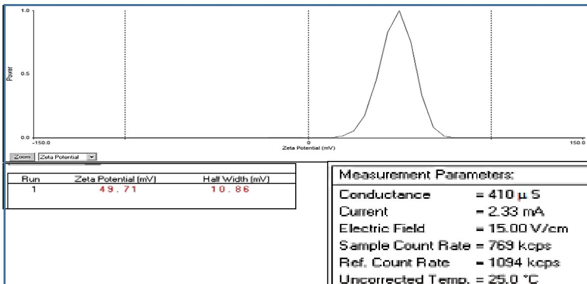
Figure 8: The zeta potential value for solution of HA/chitosan at 50 V, 6 min and 30 °C.
