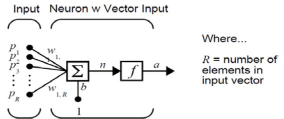
**Figure 6:** a neuron with many inputs and activation function
