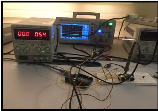
Figure 3: Sensors Connected with Arduino
