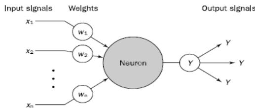
**Figure 5:** Diagram of a neural
