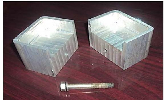
Figure 4: The die used for manufacturing composite specimen.
