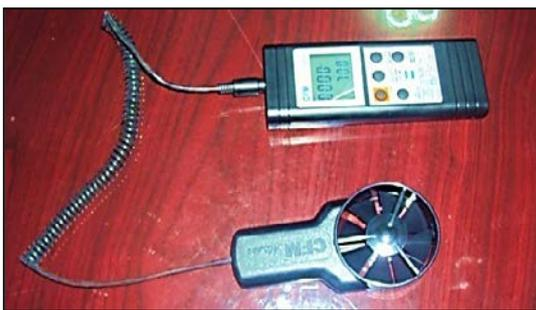
Figure 7: Anemometer device to measure the wind speed.
