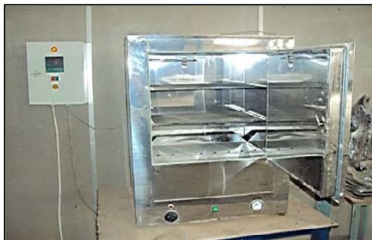
Figure 3: Furnace for manufacturing the specimens.
