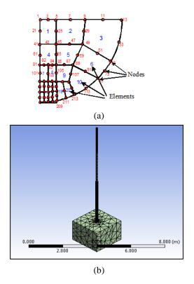
**Figure 8**: Finite element of pole. (a) 8– node element, (b) entire pole after mesh
