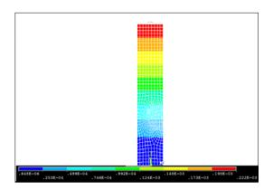
Figure 14: Deformation of composite material (m).
