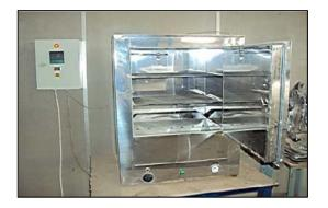
Figure 3: Furnace for manufacturing the specimens.
