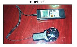
Figure 7: Anemometer device to measure the wind speed.
