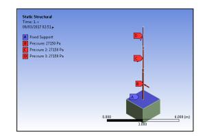
**Figure 10**: Application of loading and support of three – sections pole.
