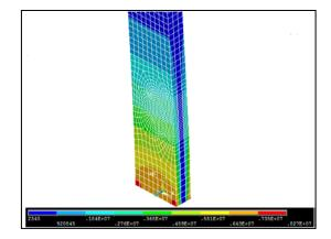
Figure 15: Von – Misses stress along 0.25 m from base  $(N/m^2)$ .
