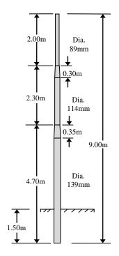
Figure 1: Three different cross section of 9 m pole length.
