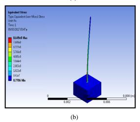
Figure 12: Von – Misses stress in pole in (Pa). (a) three sections, (b) one taper section.
