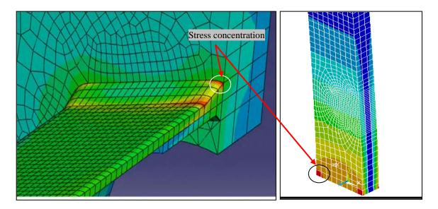
Figure 18: Stress concentration regions, (a) Results from ref [19], (b) Results of current work
