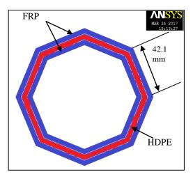
Figure 13: Octagonal cross – sectional area of pole.
