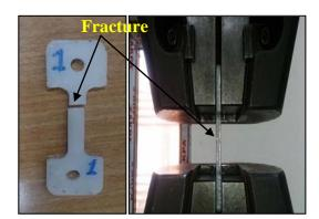
Figure 9: Fracture path of HDPE specimen caused by tensile test.
