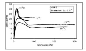
Figure 6: Effect of temperature on strength of
