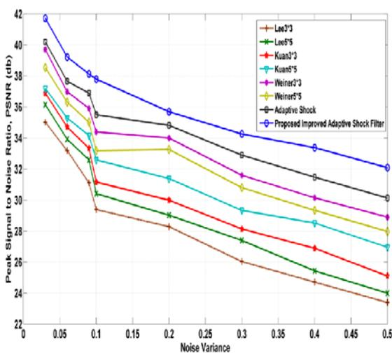
Figure 3: Performance comparison of the filters in term of PSNR.
