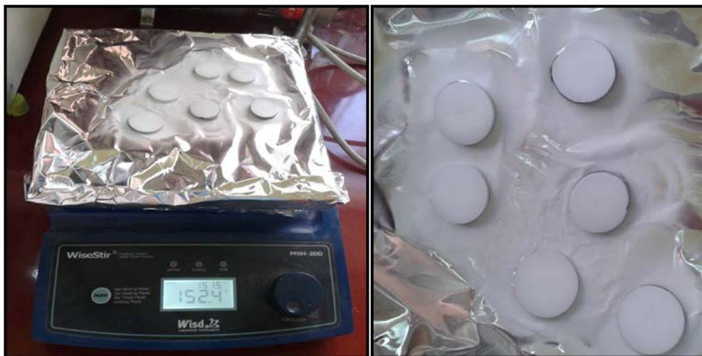
Figure 9: Coated specimens.
