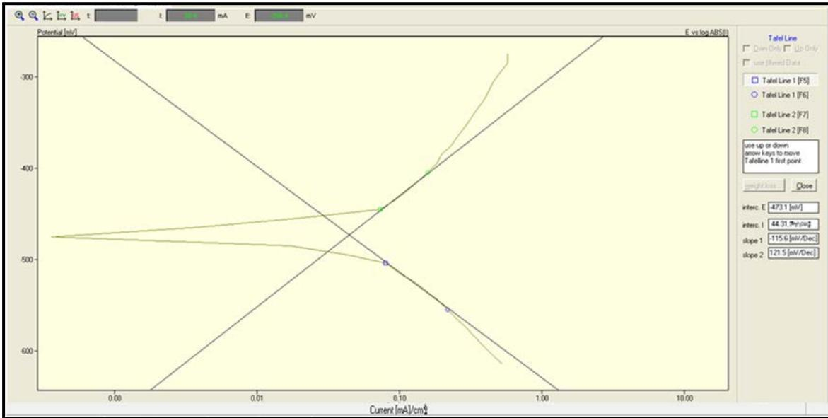
Figure 14: Tafel plot for specimen coated with (Al<sub>2</sub>O<sub>3</sub>-13 % wt TiO<sub>2</sub>).
