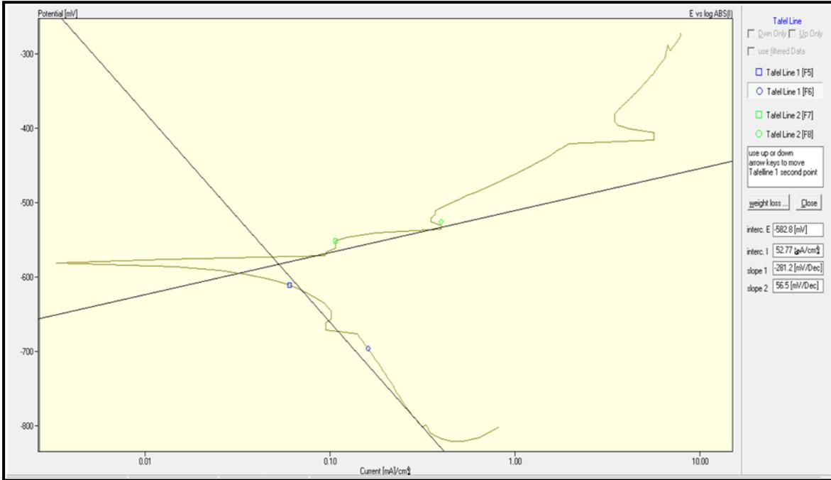
Figure 13: Tafel plot for specimen coated with (Al<sub>2</sub>O<sub>3</sub>).
