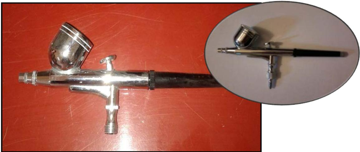
Figure 8: Airbrush device
