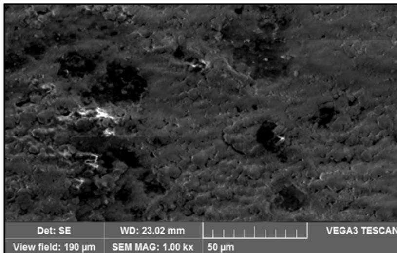
**Figure 16:** Scanning Electron Microscope image of specimen coated with (100% Al<sub>2</sub>O<sub>3</sub>) after corrosion.
