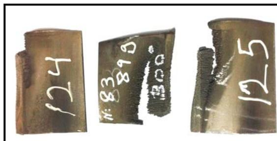
**Figure 1:** Corroded steam turbine blades
