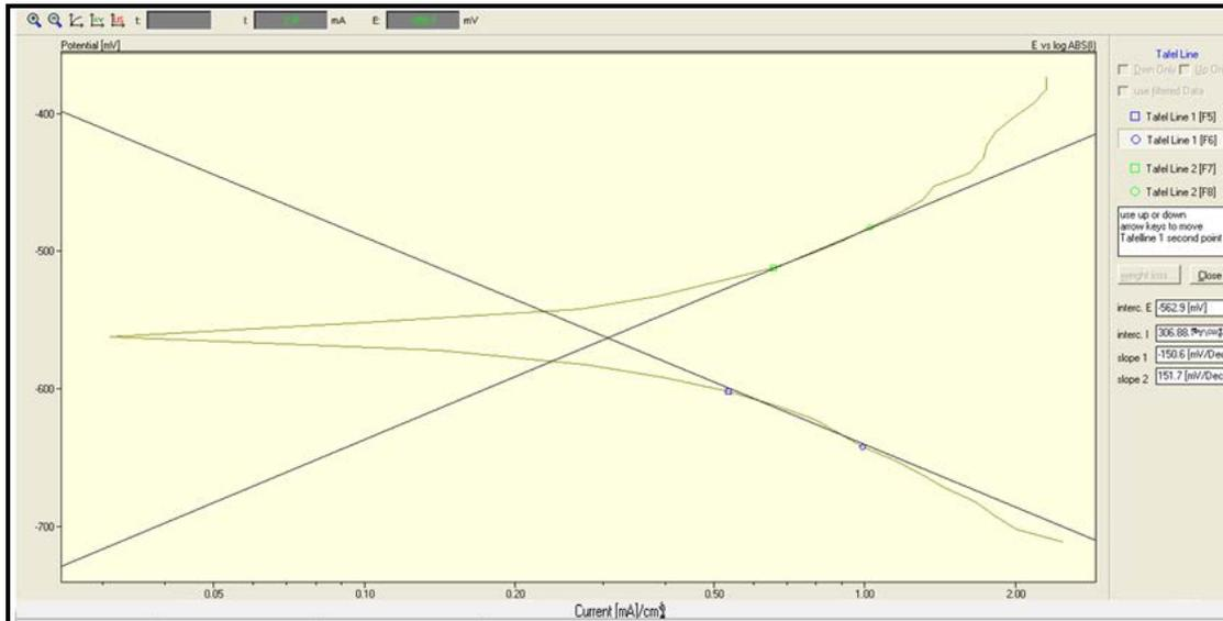
**Figure 12:** Tafel plot of uncoated specimen in 300 parts per billion Cl<sup>-</sup> and 300 parts per billion SO<sub>4</sub><sup>2-</sup> solution at 90 °C.
