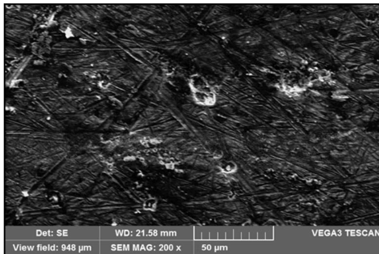
**Figure 15:** Scanning Electron Microscope image of uncoated specimen after corrosion.
