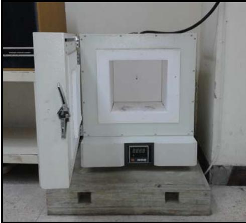
**Figure 4:** Muffle Furnace
