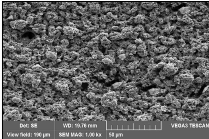
**Figure 17:** Scanning Electron Microscope image of specimen coated with (Al<sub>2</sub>O<sub>3</sub>-13 % wt TiO<sub>2</sub>) after corrosion.
