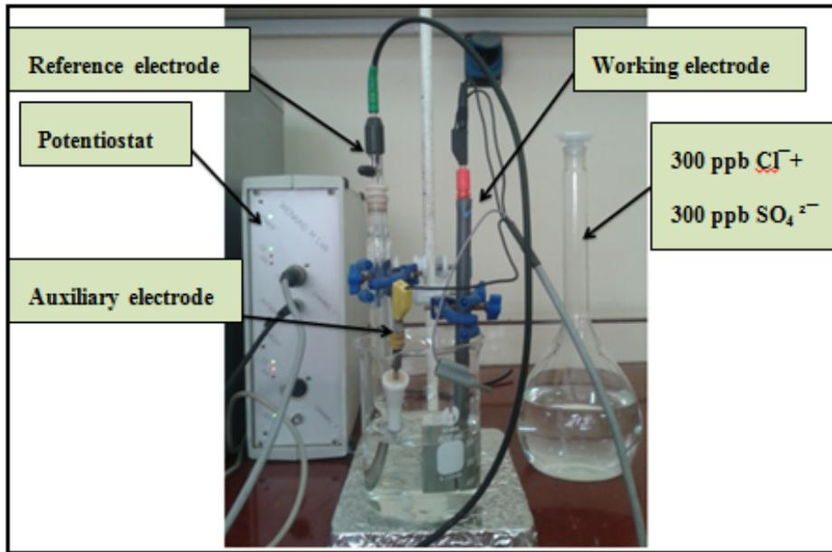
Figure 10: Corrosion cell
