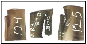
Figure 1: Corroded steam turbine blades
