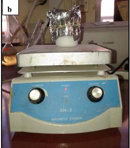
**Figure 6:** Coating solutions mixing by: (a) Ultrasonic device. (b) Magnetic mixing device
