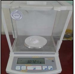
Figure 5: Sensitive balance device
