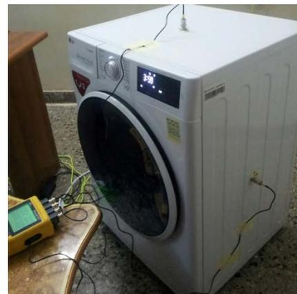
**Figure 7:** Installation locations of Vibration sensors
