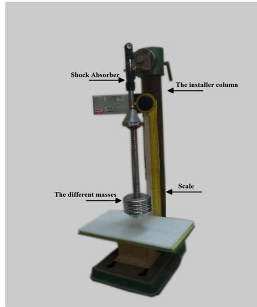
**Figure 5:** Examination device of the damping coefficient
