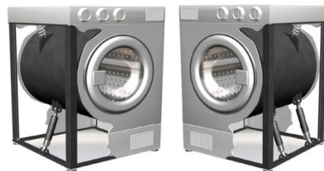
**Figure 12:** Illustration of suspension parts of washing machine
