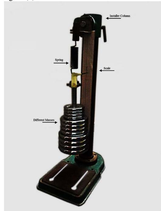
**Figure 2:** Examination device of the spring coefficient
