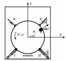
Figure 11: Physical Model of a Front load washing machine
