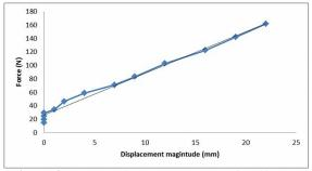
**Figure 3:** Force – displacement curve for Hinge Spring of washing machine
