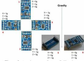
Figure 8: Accelerometer Sensor Calibration
