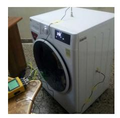
Figure 7: Installation locations of Vibration sensors
