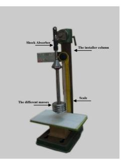
Figure 5: Examination device of the damping coefficient
