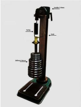
Figure 2: Examination device of the spring coefficient
