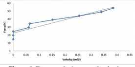
Figure 6: Force – velocity curve for shock absorber of washing machine
