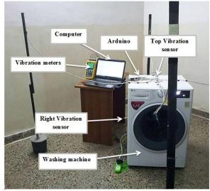
Figure 9: Building equipment for framework of washing machine
