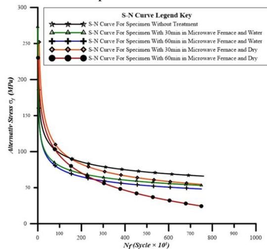
Figure 16: S – N Curves for all the Fatigue tests specimens of AA7075-T6
