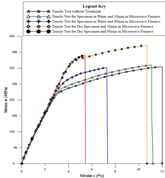
**Figure 13:** Stress – Strain diagram for tensile test of all tests specimens of AA2024-T3
