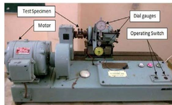
**Figure 5:** Plane Bending Fatigue Testing Machine Type Avery Model 7305
