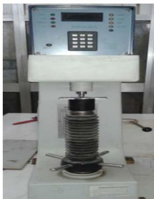
**Figure 6:** Rockwell Hardness Testing Machine
