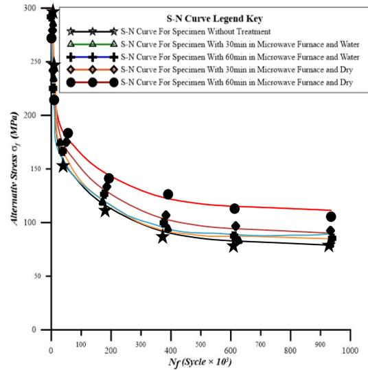
Figure 15: S – N Curves for all the Fatigue tests specimens of AA2024-T3
