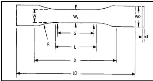
**Figure 1:** Standard Tensile Test Specimen with (T=3, LO=165, W=WC=12.5, WO=20, D=75, L=65, G=60 and R = 75, (Note that all dimensions in mm) for plane specimen [ASTM D-638-I]
