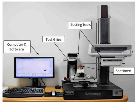
**Figure 7:** Surface Roughness Testing Machine Type Mitutoyo
