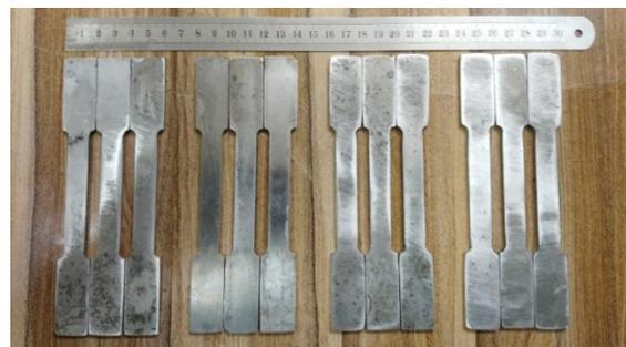
**Figure 11:** Tensile Test Specimens each three for specific test from right to left (Water 30min, Water 60min, Dry 30min and Dry 60min)
