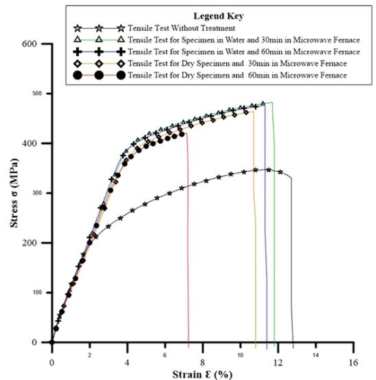
**Figure 14:** Stress – Strain diagram for tensile test of all tests specimens of AA7075-T6
