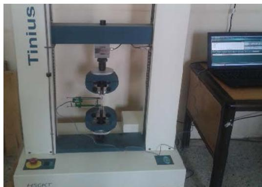
**Figure 3:** Tensile Test Machine Type Tinius Olsen
