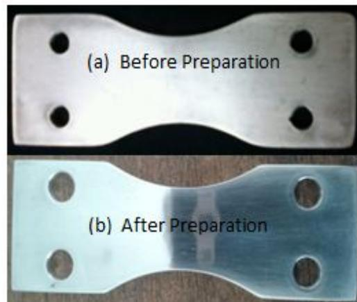
**Figure 4:** Standard Fatigue Test Specimen Preparation Steps
