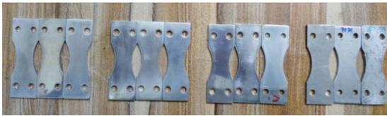
**Figure 12:** Fatigue Test Specimens each three for specific test from left to right (Water 30min, Water 60min, Dry 30min and Dry 60min)
