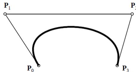
**Figure (1):** Simple Cubic Bezier curve polygon with its control points. [6]
