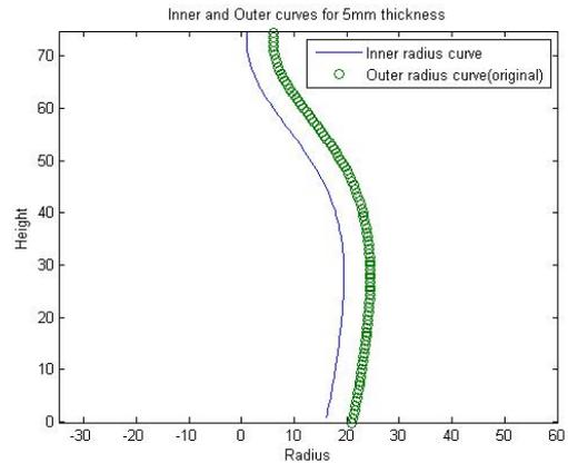
**Figure (8):** Inner and outer curves of the candle holder.
