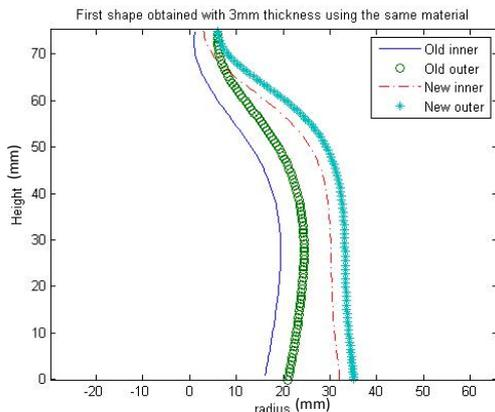
**Figure (9):** First obtained shape of the candle holder after changing the volume.
