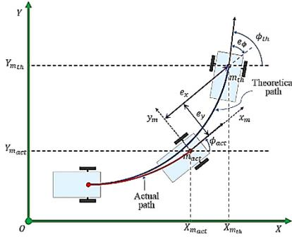
Figure 2: The position error in the local coordinate frame.
