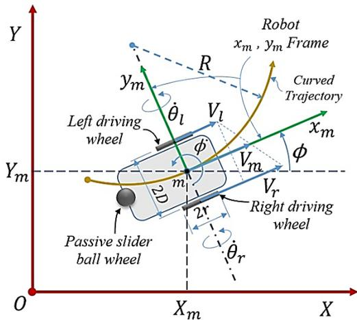
Figure 1: Kinematic structure of differential drive WMR.
