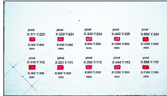
Figure 7: Positions readings (in pixel units) and actual positions (in millimetres units) of red objects.
