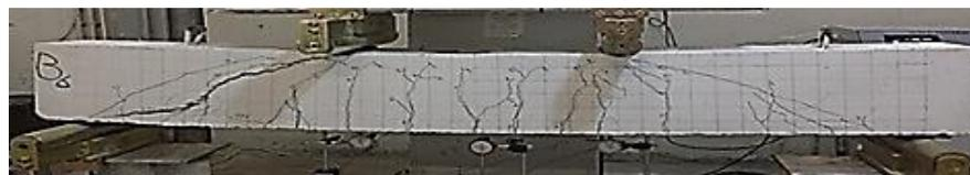
**Plate 11:** Cracks patterns in beam (B<sub>6</sub>)
