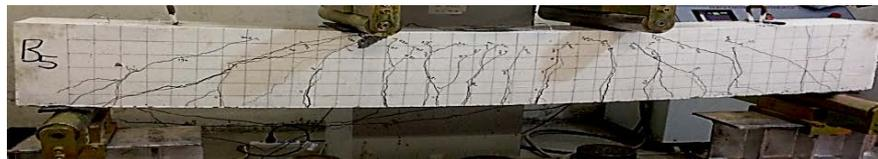
**Plate 10:** Cracks patterns in beam (B<sub>5</sub>)
