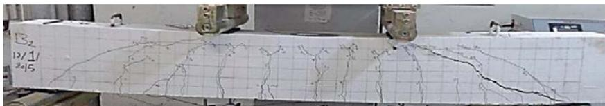
**Plate 7:** Cracks patterns in beam (B<sub>2</sub>)
