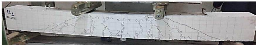
**Plate 6:** Cracks patterns in beam (B<sub>1</sub>)
