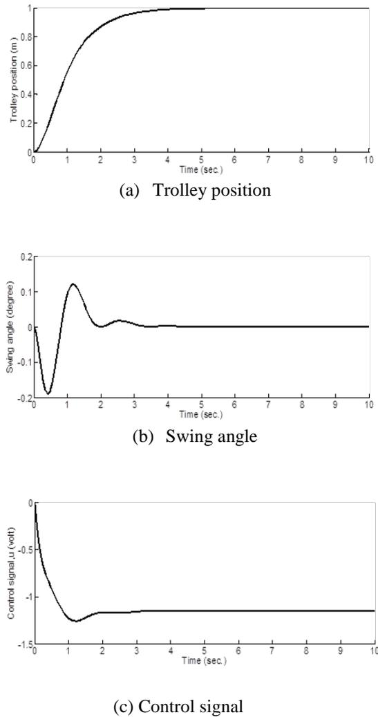
**Figure 5:** System time response with state feedback  $H_2$  control.
