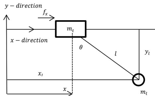
Figure 2: Overhead Crane equivalent [14].
