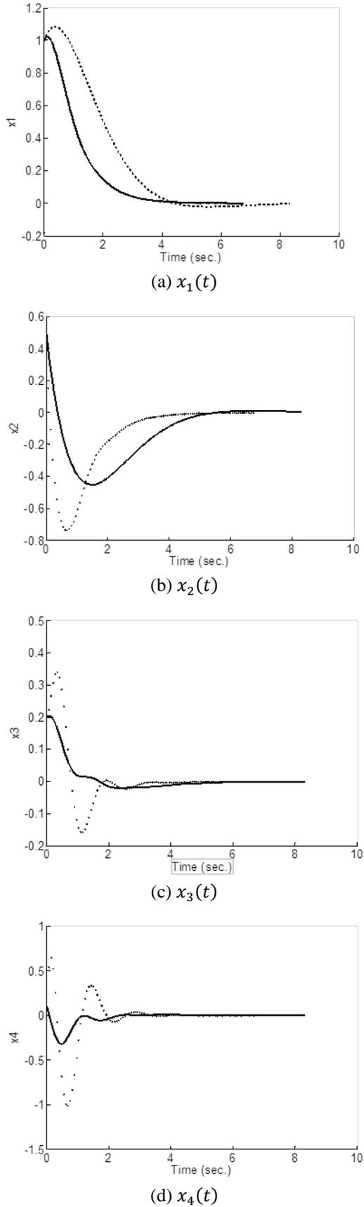
**Figure 3:** System state trajectories using state feedback  $H_2$  control (dotted line) and state derivative feedback  $H_2$  control (solid line).
