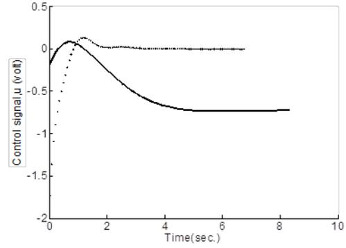
**Figure 4:** System control signal with state feedback  $H_2$  control (dotted line) and state derivative feedback  $H_2$  control (solid line)
