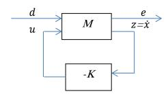
**Figure 1:** Block diagram of H<sub>2</sub> state derivative feedback [13].
