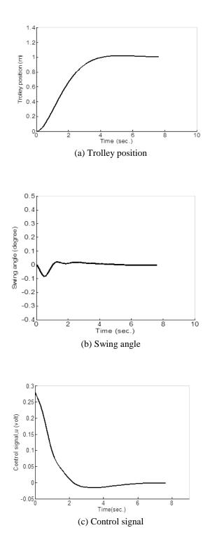
Figure 6: System time response with state derivative feedback H<sub>2</sub> control.
