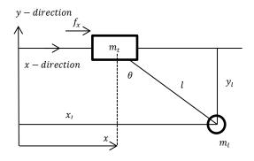
Figure 2: Overhead Crane equivalent [14].
