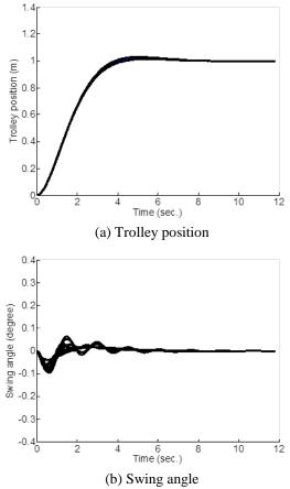
Figure 7: System time response with 50% variation in system parameters using state derivative feedback  $H_2$  control.
