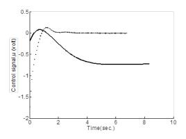
**Figure 4:** System control signal with state feedback  $H_2$  control (dotted line) and state derivative feedback  $H_2$  control (solid line)
