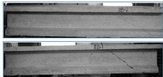
**Figure (5-B):** The crack patterns of the beams tested in the present work.
