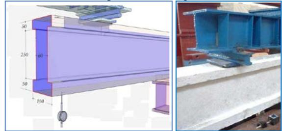
**Figure (5-A):** Reinforced Concrete I-beam under Test Machine
