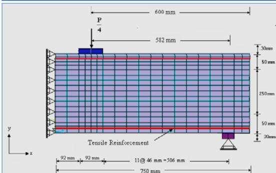
**Figure (7, b):** Typical half symmetry finite element model with dimensions (rollers as a supports at mid. Span to allow the y – direction displacement).
