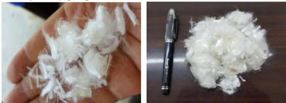
**Figure 4:** Polypropylene Fiber used in study.
