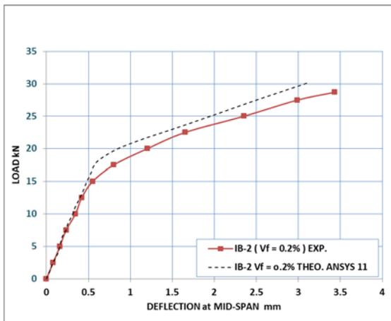
Figures (11): Comparison between Theoretical and Experimental work (load-deflection curves) at mid span IB-2.
