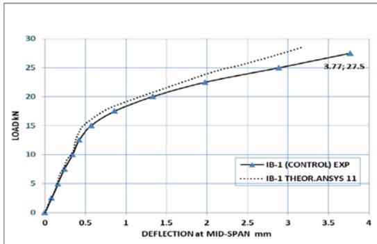
Figures (10): Comparison between Theoretical and Experimental work (load-deflection curves) at mid span for IB-1.
