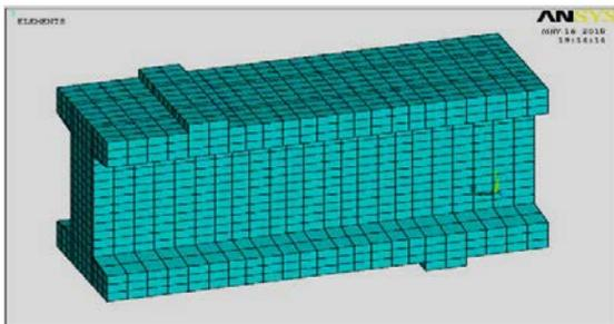
**Figure (7, a):** Typical half symmetry finite element model.
