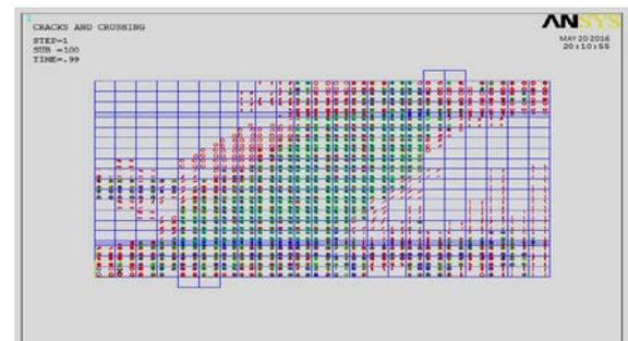
**Figure 8:** Crack Pattern of PPFRC IB-1 (ANSYS 11)
