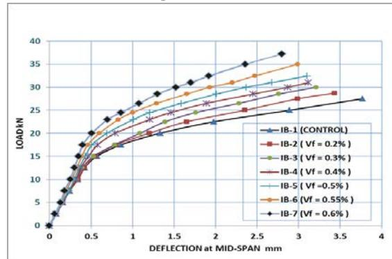
**Figure 6:** Load – Deflection curves for experimental work.
