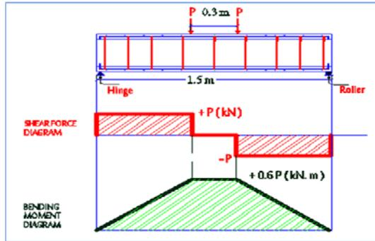
Figure 2: shear force and bending moment diagrams.
