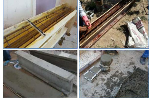
Figure 3: Preparing Specimens for Casting.
