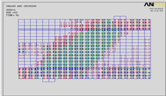
Figure 9: Crack Pattern of PPFRC IB-2 (ANSYS 11).
