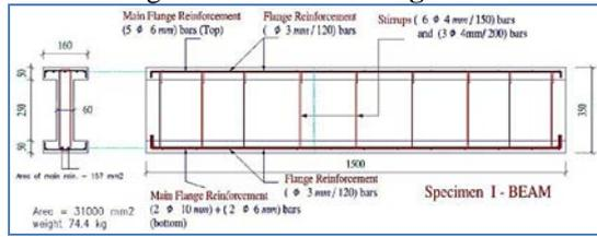
Figure 1: Geometry and Sectional Dimensions of the I-section Reinforced Concrete Beam (units: mm)
