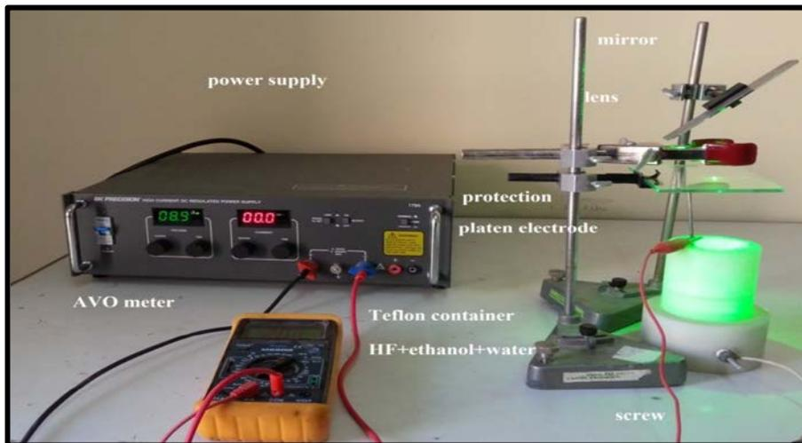
Figure (4): Photographic image of PECE system.
