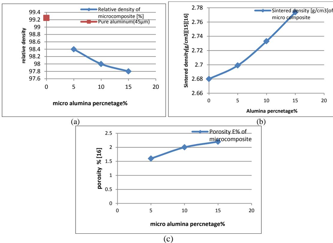
**Figure 1:** Aluminum and micro alumina reinforcement in Microcomposites AMMC (a) relative density (b)sintered density (c) Porosity
