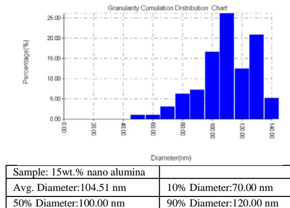
**Figure 13 :** Granularity accumulation distribution graphs and diameters percentage for composites with an additives of (a)- 5wt.% nano alumina (b)- 15wt.% nano alumina
