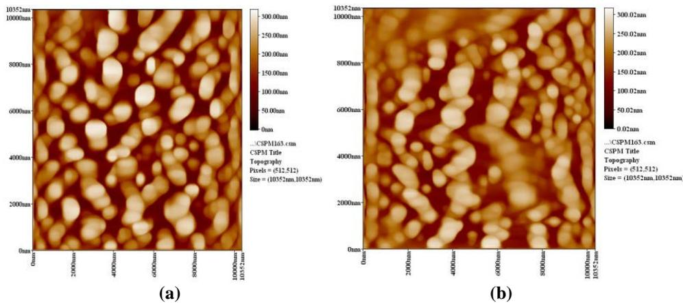
**Figure 4 :** AFM pictures with 10000 nano meter magnification for aluminum with (a) 5wt.% micro alumina (b) 15wt.% micro alumina
