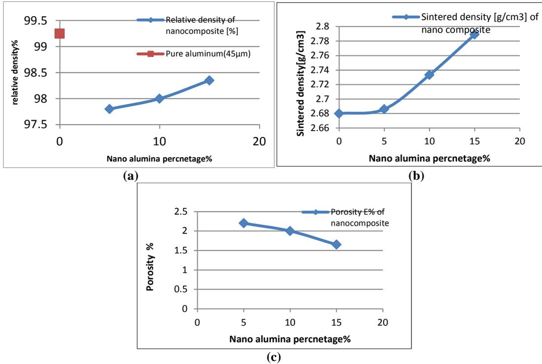
**Figure 2:** Aluminum and nano alumina reinforcement in Nanocomposites AMMC (a) relative density (b)sintered density (c) Porosity
