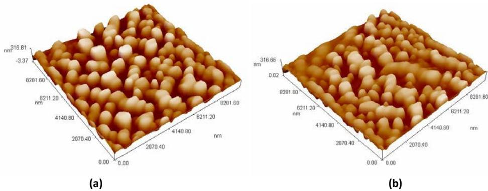
**Figure 5 :** Three dimensional (XYZ) AFM pictures with 10000 nano meter magnification for aluminum with (a) 5wt.% micro alumina (b) 15wt.% micro alumina
