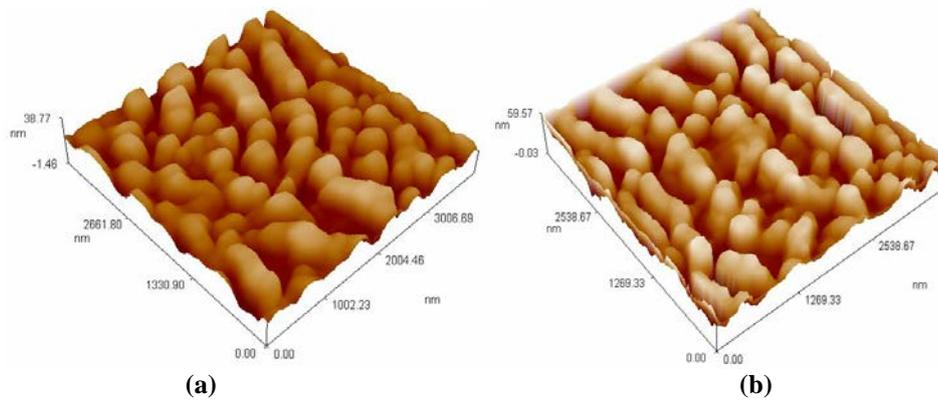
**Figure 7:** Three dimensional (XYZ) AFM pictures with 4000 nano meter magnification for aluminum with (a) 5%wt. micro alumina (b) 15wt.% micro alumina
