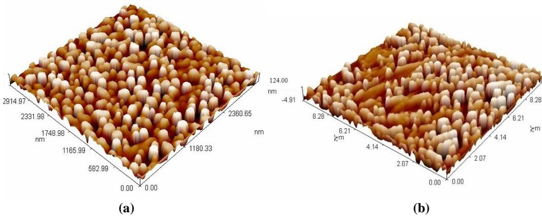
**Figure 12 :** Three dimensional (XYZ) AFM pictures with 4000 nano meter magnification for aluminum matrix with (a) 5% wt. nano alumina (b) 15% wt. nano alumina
