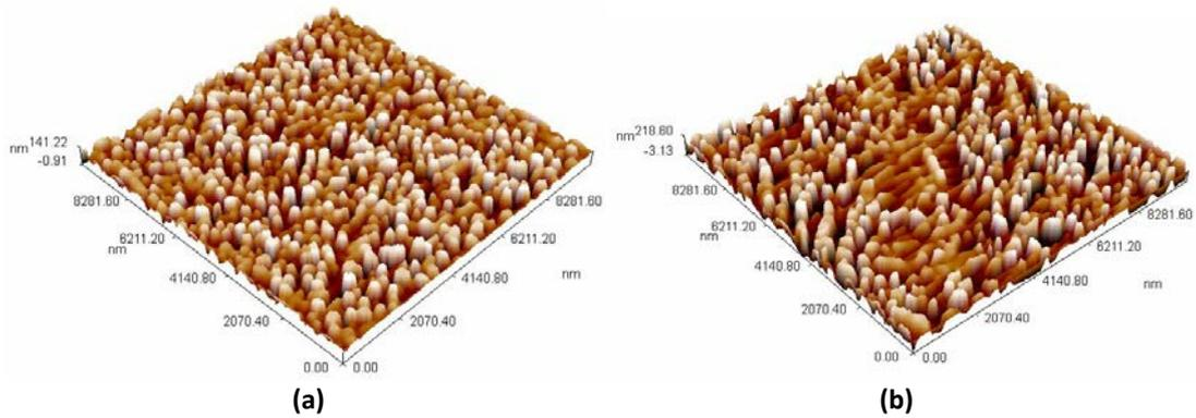
**Figure 10 :** Three dimensional (XYZ) AFM pictures with 10000 nano meter magnification for aluminum matrix with (a) 5% wt. nano alumina (b) 15% wt. nano alumina
