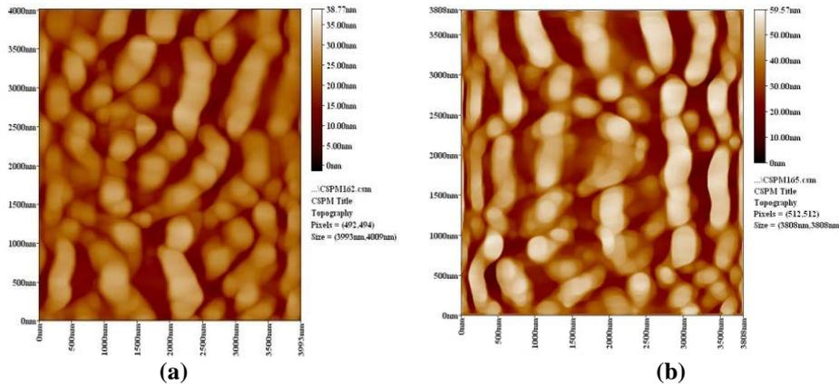
**Figure 6:** AFM pictures with 4000 nano meter magnification for aluminum with (a) 5wt.% micro alumina (b) 15wt.% micro alumina
