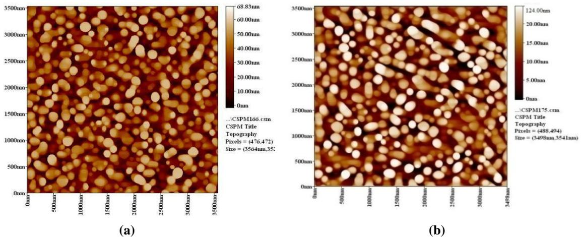
**Figure 11 :** AFM pictures with 4000 nano meter magnification for aluminum matrix with (a) 5% wt. nano alumina N1 (b) 15% wt. nano alumina N3
