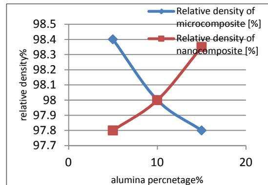
**Figure 3:** Relative densities variation according to the amount of alumina wt.% in micro composite and nano composite
