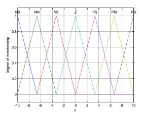
**Figure 6**: I/O Membership functions of FLC. Table (2). FLC rules table.
