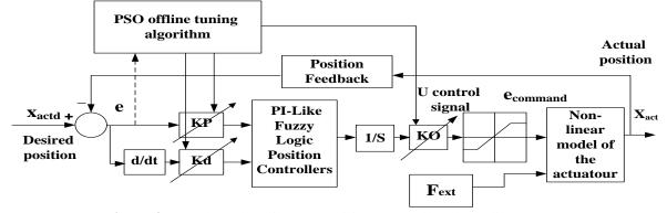
Figure 9: PSO-based PI-like FL Position Controller block diagram.
