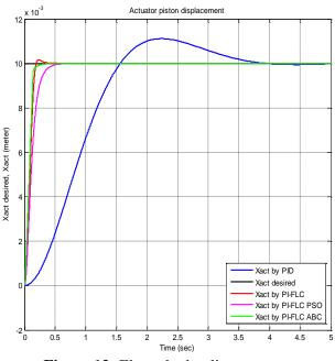
Figure 12: Electrohydraulic servo-actuator position response by conventional and intelligent controllers.
