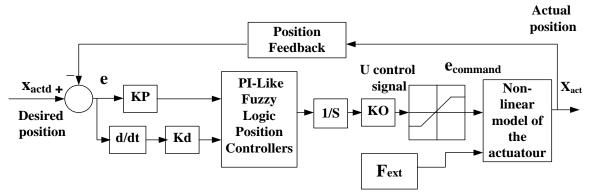
Figure 4: block diagram of controlled actuator by PI-FLC.
