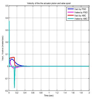
Figure 15: Actuator piston velocity with valve spool velocity by PI-FLC based on PSO and ABC.
