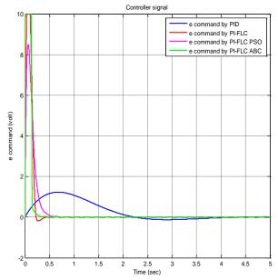
Figure 13: . Control signal of conventional and intelligent controllers to matching the desired position.
