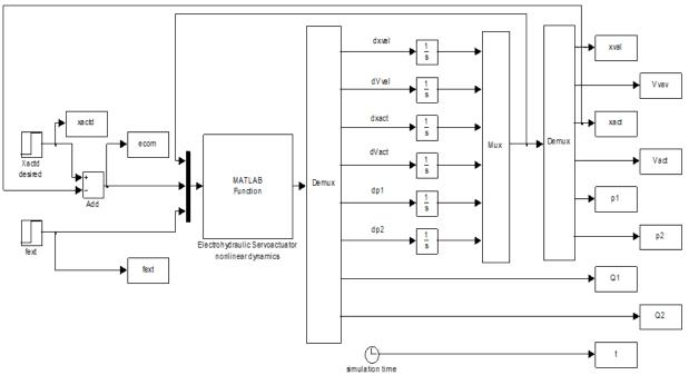
Figure (3). Electrohydraulic Servo-actuator Simulink model.
