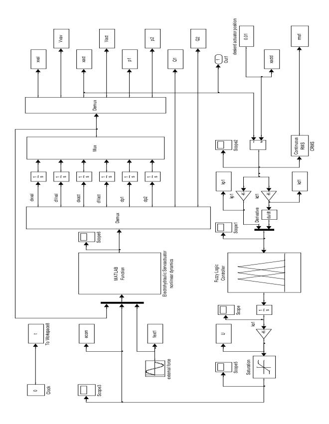
Figure 7: Simulink model of PI-like FLC with actuator model blocks.
