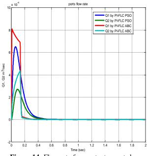
Figure 14: Flow rate from actuator ports by PI-FLC based on PSO and ABC.
