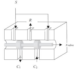
Figure2: The valve spool and ports.
