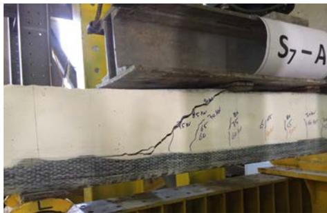
(b) Cracking pattern at failure for beam S7-A, Experimental test
