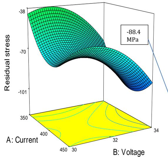
**Figure (10):** The minimum residual stress at the optimum welding parameters (welding current of 450 amp., arc voltage of 34 volt, welding speed of 38 cpm, and included angle of 60°)
