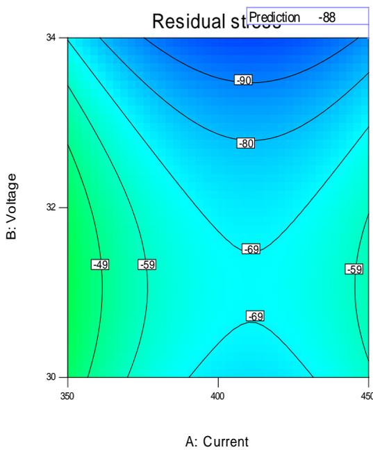
**Figure (9):** The minimum residual stress at the optimum welding parameters (welding current of 450 amp. arc voltage of 34 volt, welding speed of 38 cpm, and included angle of 60°).
