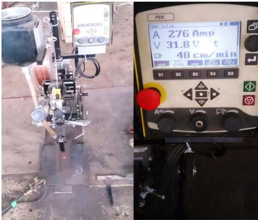
**Figure (2):** EsabA2 Multitrack with the A2-A6 process controller PEK
