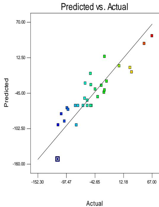
**Figure (5):** Predicted versus actual residual stress data for comparison
