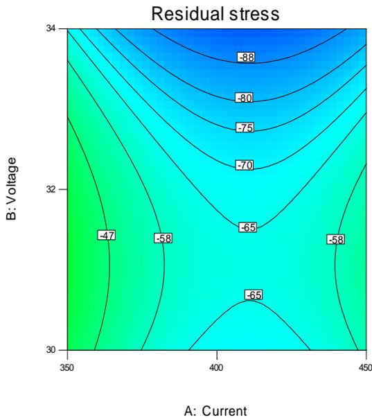
**Figure (7):** 2D plot of residual stress as a function at center level of welding speed (40 cpm) and included angle (60°).
