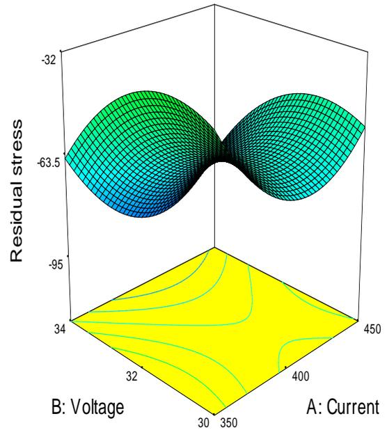
**Figure (8):** 3D plot plot of residual stress at a function at center level of welding speed (40 cpm) and included angle (60°).
