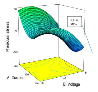
**Figure (10):** The minimum residual stress at the optimum welding parameters (welding current of 450 amp., arc voltage of 34 volt, welding speed of 38 cpm, and included angle of  $60^{\circ}$ )
