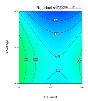
**Figure (9):** The minimum residual stress at the optimum welding parameters (welding current of 450 amp. arc voltage of 34 volt, welding speed of 38 cpm, and included angle of 60°).
