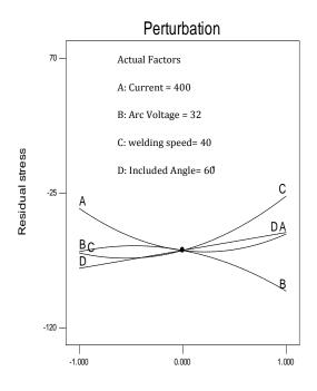
Deviation from Reference Point (Coded Units) **Figure (6):** Perturbation of residual stress showing the effect of each input parameter over the selected level.
