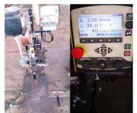
Figure (2): EsabA2 Multitrack with the A2-A6 process controller PEK
