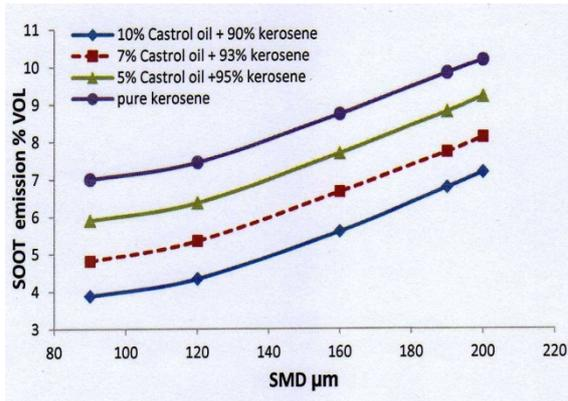
Figure 21: Soot emission from kerosene bio-blend vs. SMD at  $\phi = 1$
