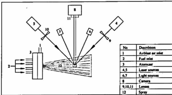
Figure 4: Droplet size measurement system [7].
