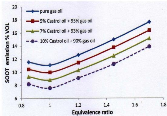
Figure 12: Soot emission from gasoil bio-blend vs. equivalence ratio with SMD=100  $\mu\text{m}$ .
