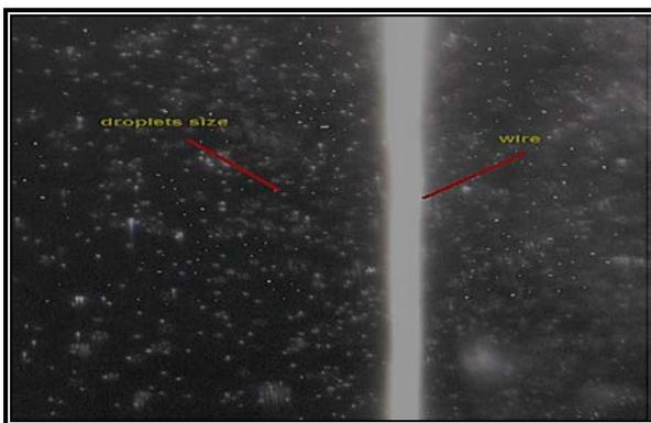
Figure 5: Photograph of the spray captured by the camera for comparison between wire and droplets (SMD = 100 μm).
