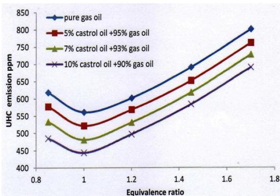
Figure 8: UHC emission from gasoil bio-blend vs. equivalence ratio with SMD=100  $\mu\text{m}$ .
