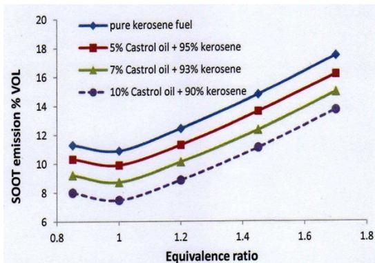
Figure 13: Soot emission from kerosene bio-blend vs. equivalence ratio with SMD=100  $\mu\text{m}$ .
