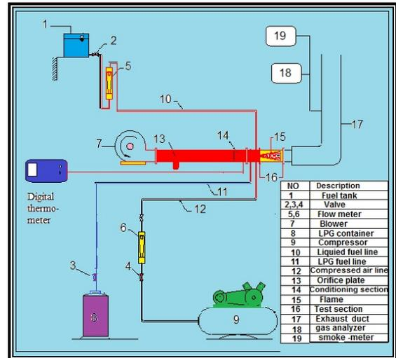
Figure 1: The test rig.
