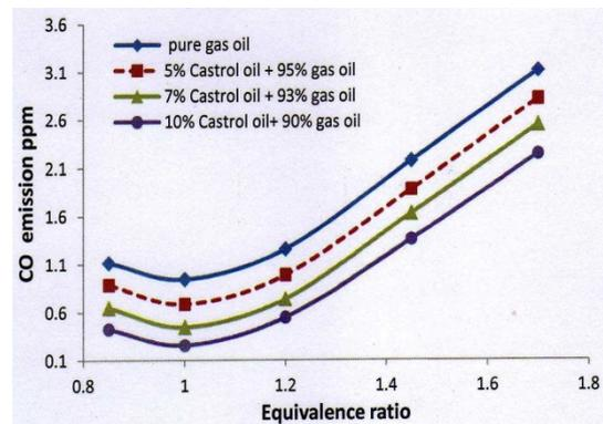
Figure 6: CO emission from gasoil bio-blend vs. equivalence ratio with SMD=100 μm.
