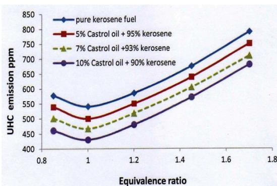
Figure 9: UHC emission from kerosene bio-blend vs. equivalence ratio with SMD=100  $\mu\text{m}$
