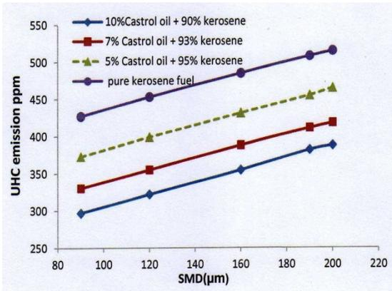
Figure 17: UHC emission from kerosene bio-blend vs. SMD at  $\phi = 1$
