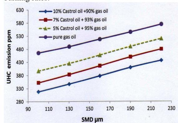
Figure 16: UHC emission from gasoil bio-blend vs. SMD at  $\phi = 1$
