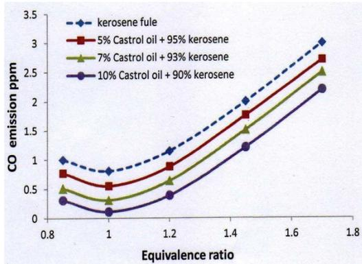
Figure 7: CO emission from kerosene bio-blend vs. equivalence ratio with SMD=100  $\mu\text{m}$
