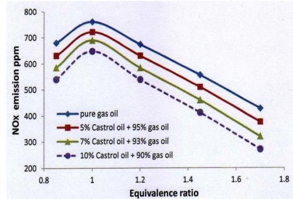
Figure 10:  $\text{NO}_x$  emission from gasoil bio-blend vs. equivalence ratio with SMD=100  $\mu\text{m}$ .
