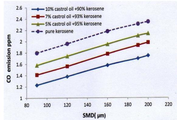
Figure 15: CO emission from kerosene bio-blend vs. SMD at  $\phi = 1$
