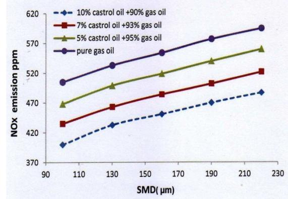
Figure 18:  $\text{NO}_x$  emission from gasoil bio-blend vs. SMD at  $\phi = 1$
