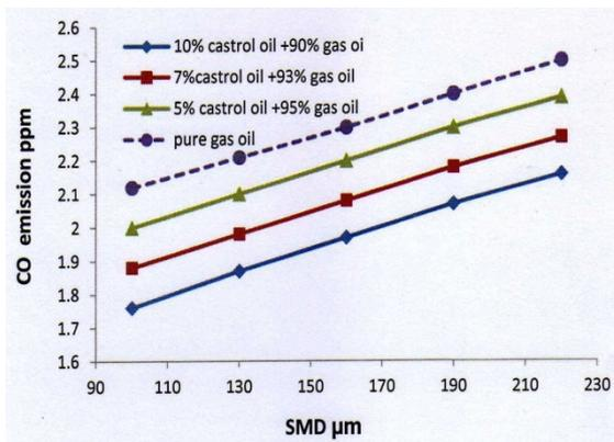
Figure 14: CO emission from gasoil bio-blend vs. SMD at  $\phi = 1$
