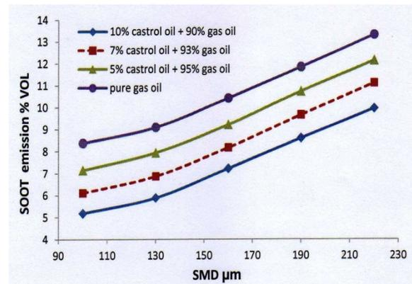
Figure 20: Soot emission from gasoil bio-blend vs. SMD at  $\phi = 1$
