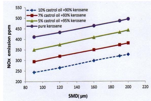
Figure 19:  $\text{NO}_x$  emission from kerosene bio-blend vs. SMD at  $\phi = 1$
