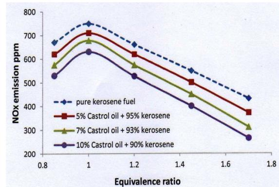
Figure 11:  $\text{NO}_x$  emission from kerosene bio-blend vs. equivalence ratio with SMD=100  $\mu\text{m}$
