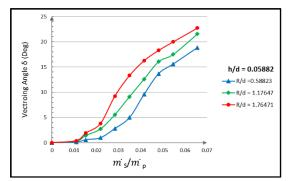
**Figure 12:** Experimental results of Thrust vectoring angle for varying Coanda surface radius at constant secondary gap height h/d = 0.05882
