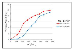
**Figure 16:** Numerical results of Thrust vectoring angle for varying secondary gap height at constant Coanda surface radius R/d = 1.17647
