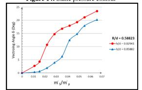
**Figure 15:** Numerical results of Thrust vectoring angle for varying secondary gap height at constant Coanda surface radius R/d = 0.58823
