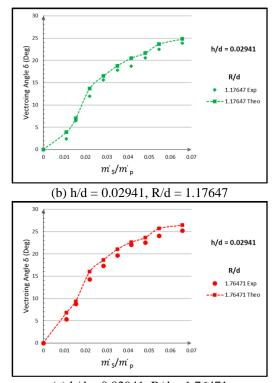
(c) h/d = 0.02941, R/d = 1.76471Figure 21: Comparison between theoretical and experimental results for varying Coanda radius at constant secondary gap height h/d = 0.02941
