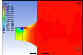
R/d = 1.76471, h/d = 0.02941,  $\dot{m}_s/\dot{m}_p = 0.06568$ Figure 14: Static pressure contour
