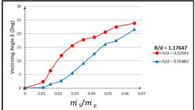
**Figure 8:** Experimental results of Thrust vectoring angle for varying secondary gap height at constant Coanda surface radius R/d = 1.17647
