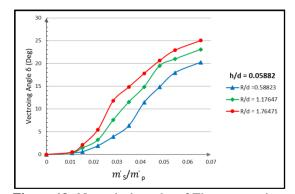
**Figure 19:** Numerical results of Thrust vectoring angle for varying Coanda surface radius at constant secondary gap height h/d = 0.05882
