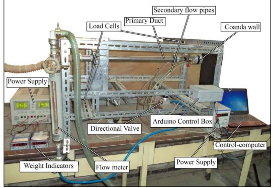
Figure 5: Photograph of the experimental rig
