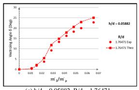
(c) h/d = 0.05882, R/d = 1.76471Figure 22: Comparison between theoretical and experimental results for varying Coanda radius at constant secondary gap height h/d = 0.05882
