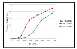
**Figure 7:** Experimental results of Thrust vectoring angle for varying secondary gap height at constant Coanda surface radius R/d = 0.58823
