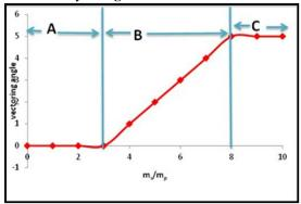
**Figure 10:** Trend line of the experimental results: A – Dead zone, B – Active control, C – Saturation
