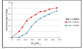
**Figure 9:** Experimental results of Thrust vectoring angle for varying secondary gap height at constant Coanda surface radius R/d = 1.76471
