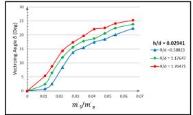
**Figure 11:** Experimental results of Thrust vectoring angle for varying Coanda surface radius at constant secondary gap height h/d = 0.02941
