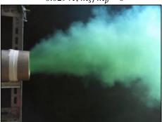
(b) Vectored primary flow, R/d =1.76471, h/d = 0.02941,  $\dot{m_s}/\dot{m_p} = 0.06568$ Figure 20: Smoke visualization of a vectored and non-vectored primary jet
