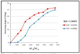
**Figure 17:** Numerical results of Thrust vectoring angle for varying secondary gap height at constant Coanda surface radius R/d = 1.76471
