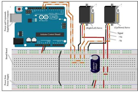
Figure 6: Schematic of the Arduino board valve control circuit
