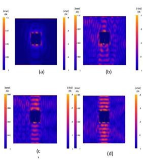
**Figure 12:** Current and electric field distribution for capacitively-fed RPMA at, frequencies, f, :(a)1.9,(b)2.76,(c)2.92and (d)3.24GHz
