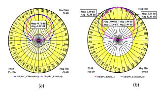
**Figure 5:** (a) Maximum radiation at 0dB and (b) HPBW at -3dB for both principal planes at f=2.15 GHz for thin substrate RPMA
