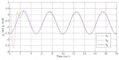
Figure 4: Position performances for joints 1 and 2 tracking desired trajectory.
