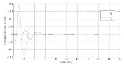
Figure 5: Position tracking errors for joints 1 and 2 against desired trajectory.
