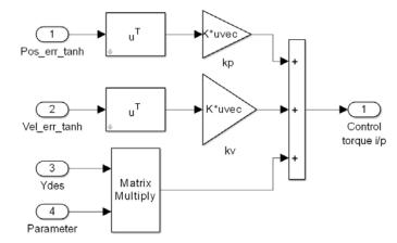
Figure A4: Control law represented in Matlab/Simulink Block diagram.
