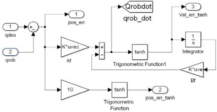
Figure A2: Velocity estimator represented in Matlab/Simulink Block diagram.
