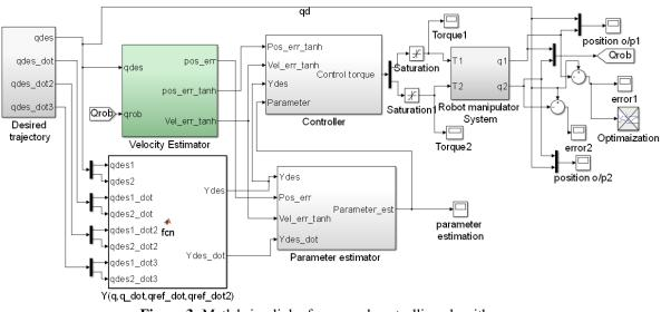
Figure 3: Matlabsimulink of proposed controlling algorithm.
