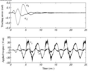
Figure 9: The tacking error and applied torques obtained by using controller presented by references [2] and [3].
