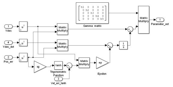
Figure A3: Parameters estimation represented in Matlab/Simulink Block diagram.
