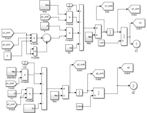
Figure A1: 2-link robot manipulator modelled in Matlab/Simulink Block diagram.
