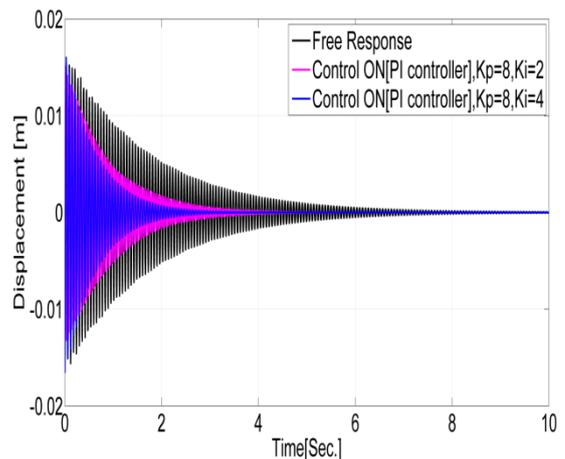
**Figure 19:** Comparison of numerically measured responses for aluminium foam triangular wing with PI controller.
