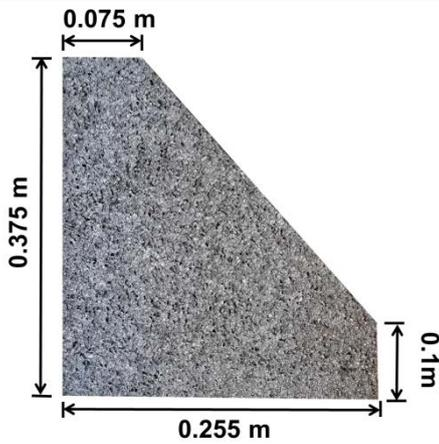
Figure 6: Typical aluminium foam delta wing
