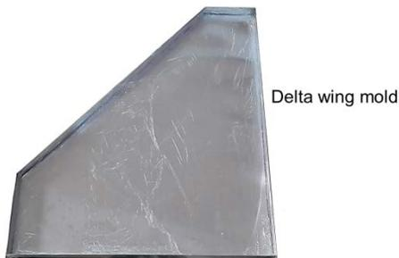
Figure 7: Mold for composite delta wing
