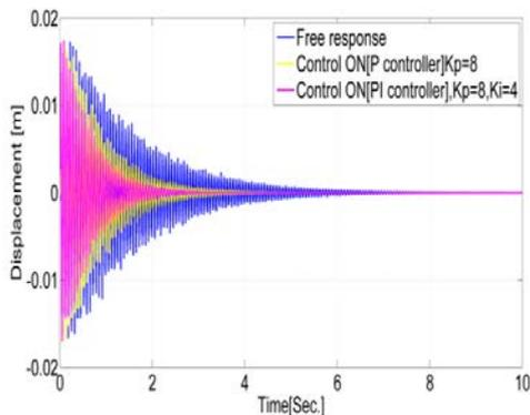
**Figure 22:** Comparison of experimentally measured responses for aluminium foam delta wing with P, PI controller.
