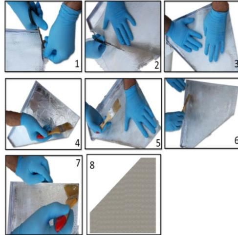
Figure 8: Manufacturing process of composite delta wing
