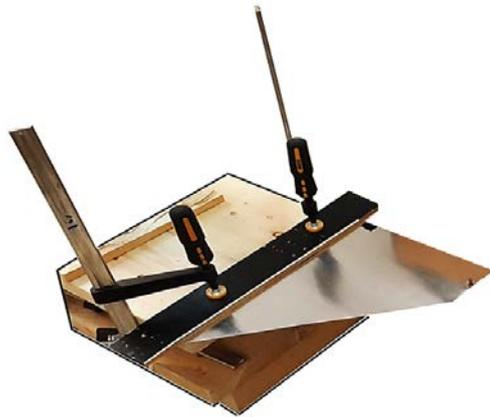
**Figure 10:** Boundary condition of delta wing
