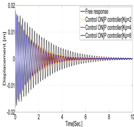
**Figure 16:** Comparison of numerically measured responses for Composite triangular wing with p controller.
