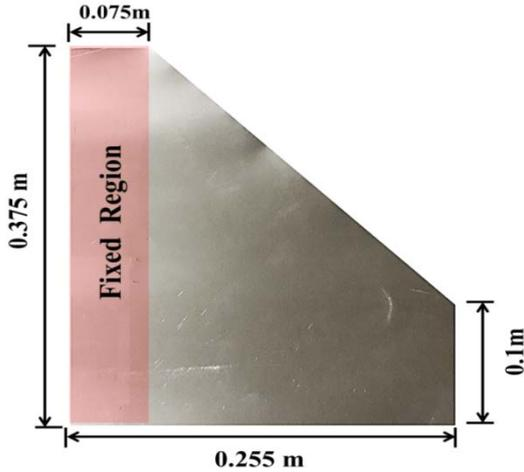
Figure 5: Typical Aluminium delta wing
