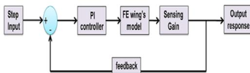
Figure 1: Block diagram of PI controlling loop
