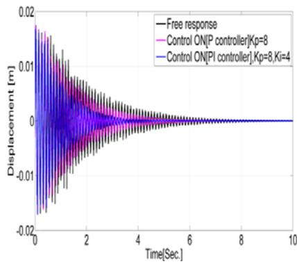
**Figure 21:** Comparison of experimentally measured responses for composite delta wing with P, PI controller.
