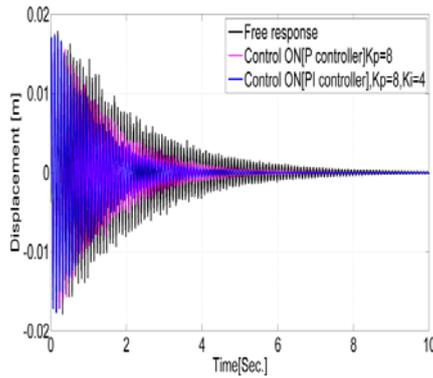
**Figure 20:** Comparison of experimentally measured responses for aluminium delta wing with P, PI controller.
