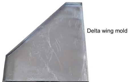
Figure 7: Mold for composite delta wing
