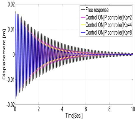
**Figure 14:** Comparison of numerically measured responses for Aluminium triangular wing with P controller.
