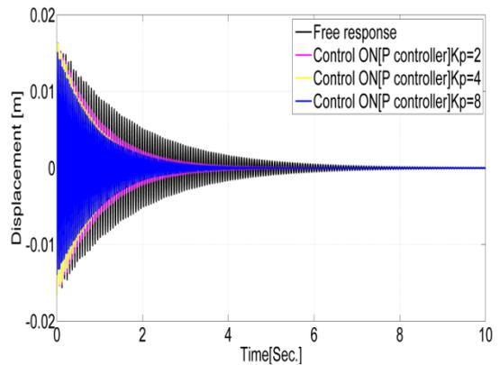
**Figure 18:** Comparison of numerically measured responses for aluminium foam triangular wing with P controller.
