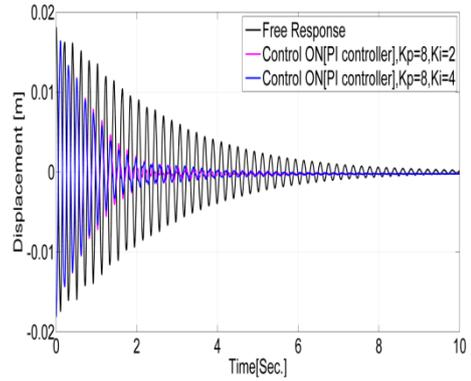
**Figure 17:** Comparison of numerically measured responses for Composite triangular wing with PI controller.
