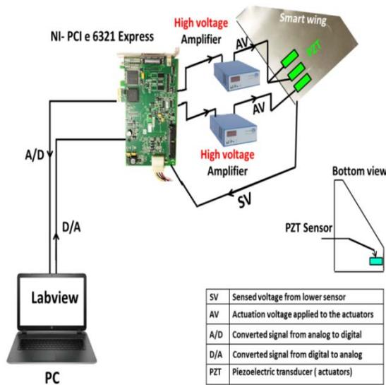
**Figure 12:** Schematic view of the experimental active vibration control setup – Delta wing
