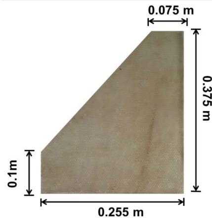
Figure 9: Typical [0/90] composite delta wing
