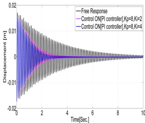
**Figure 15:** Comparison of numerically measured responses for Aluminium triangular wing with PI controller.
