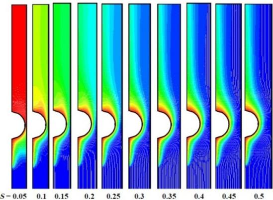
Figure (9) Temperature contour with various spacing between the tube for ( $Ra=10^5$ ,  $Pr=0.7$ , and tube position  $\delta=0.75$ )
