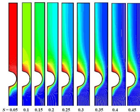
Figure (7) Temperature contour with various spacing between the tube for ( $Ra=10^5$ ,  $Pr=0.7$ , and tube position  $\delta=0.25$ )
