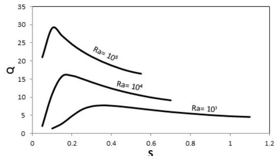
Figure (10) Heat Transfer Density with spacing at different Rayleigh numbers for tube position ( $\delta = 0.25$ )
