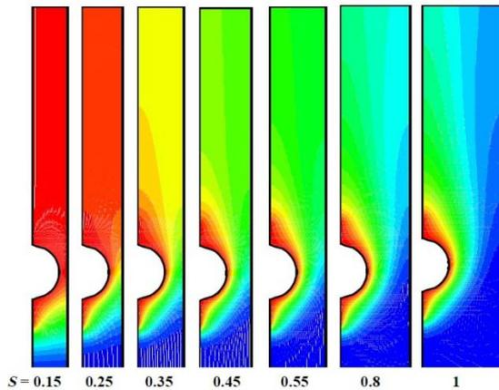
Figure (6) Temperature contour with various spacing between the tube for ( $Ra=10^3$ ,  $Pr=0.7$ , and tube position  $\delta=0.5$ )
