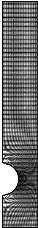
Figure (3) Generated Grid for CVs (175X50)
