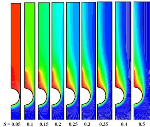
Figure (5) Temperature contour with various spacing between the tube for ( $Ra=10^5$ ,  $Pr=0.7$ , and tube position  $\delta=0.25$ )
