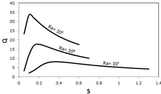
Figure (11) Heat Transfer Density with spacing at different Rayleigh numbers for tube position ( $\delta = 0.75$ )
