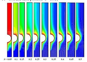
Figure (9) Temperature contour with various spacing between the tube for (Ra= $10^5$ , Pr =0.7, and tube position  $\delta$ =0.75)
