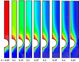
Figure (7) Temperature contour with various spacing between the tube for (Ra= $10^5$ , Pr =0.7, and tube position  $\delta$ =0.25)
