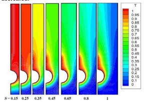
Figure (4) Temperature contour with various spacing between the tube for (Ra= $10^3$ , Pr =0.7, and tube position  $\delta$ =0.25)
