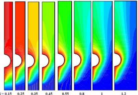
Figure (8) Temperature contour with various spacing between the tube for (Ra= $10^3$ , Pr =0.7, and tube position  $\delta$ =0.75)
