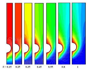
Figure (6) Temperature contour with various spacing between the tube for  $(Ra=10^3, Pr=0.7,$
