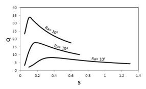
Figure (11) Heat Transfer Density with spacing at different Rayleigh numbers for tube position ( $\delta$  =0.75)
