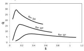
Figure (10) Heat Transfer Density with spacing at different Rayleigh numbers for tube position ( $\delta$  =0.25)
