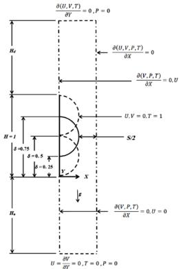
**Figure** (2): Dimensionless Boundary Conditions on the Flow Channel
