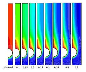
Figure (5) Temperature contour with various spacing between the tube for (Ra= $10^5$ , Pr =0.7, and tube position  $\delta$ =0.25)
