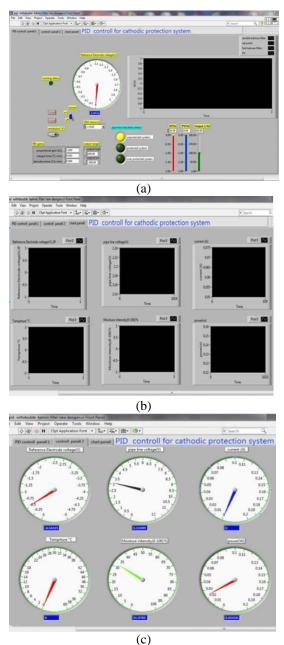
**Figure 5:** LabVIEW HMI design for the PID closed loop system; (a) front panel and (b) Time graphs panel for the measured parameters and (c) meters panel.
