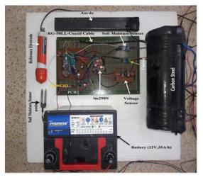
Figure 2: The built ICCP system components.
