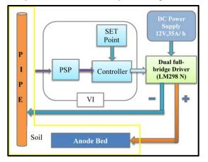
Figure 3: The ICCP system block diagram.
