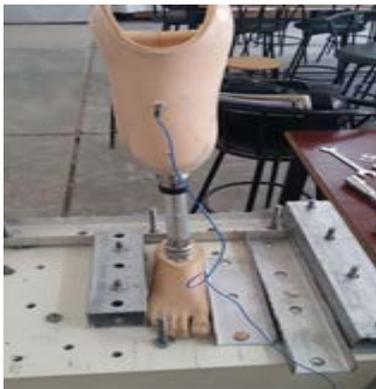
Figure 4: Prosthesis leg at support phase test
