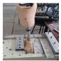
Figure 4: Prosthesis leg at support phase test
