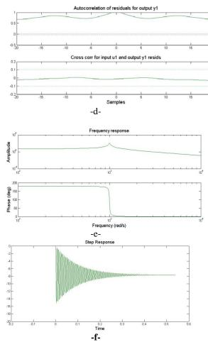
Figure 8: SID plots of prosthesis at swing phase
