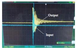
Figure 6: Real input and output wave signals for beam
