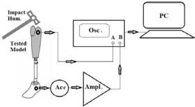
**Figure 5:** Block diagram of measuring equipment used in Prosthetics leg tests
