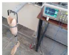
Figure 3: Prosthesis leg at swing phase test
