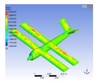
Figure 6: The comparison of Lift force between the two models.
