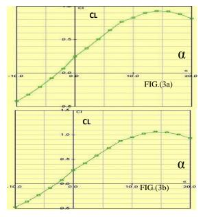
**Figure 3:** Relationship between Lift coefficient (CL) & angle of attack ( $\alpha$ ) from Java Foil
