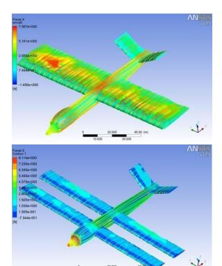
Figure7: The comparison of Drag force between the two models.
