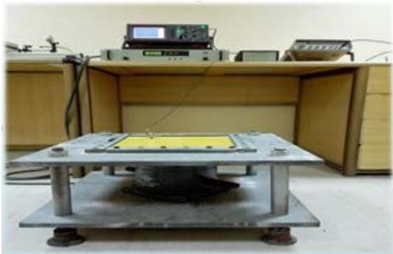
Figure (1): set up for modal testing of a laminated plate
