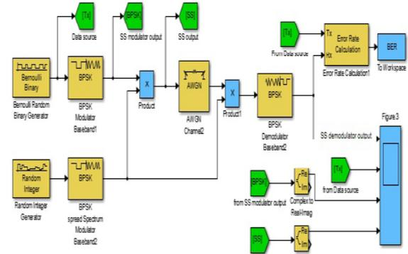
**Figure.2** Simulink model of DSSS using BPSK modulation
