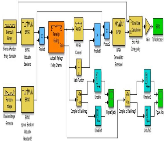
**Figure.4** Simulink model of Non-quantized DSSS with Rayleigh fading channel
