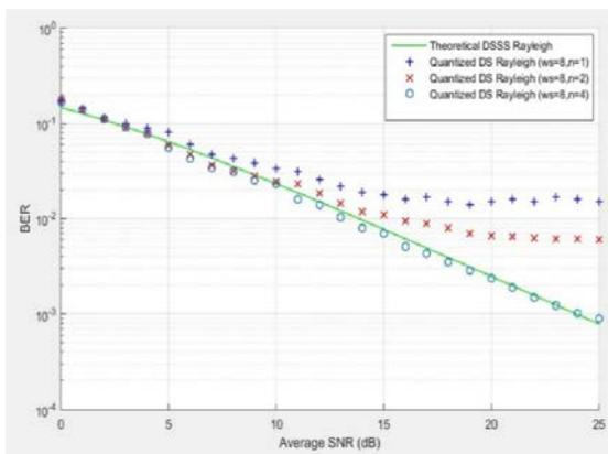
Figure.12 BER performance of Quantized DSSS with Rayleigh channel for different quantization levels
