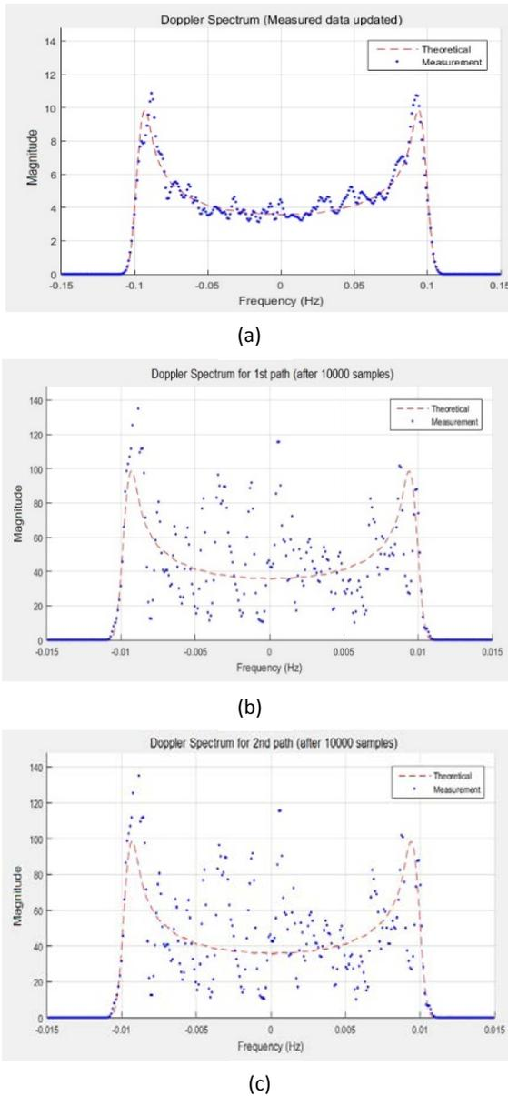
**Figure.14** Rician channel Doppler spectrum for Rician factor=3 and after 10000 samples: (a) Doppler spectrum without multipath, (b) Doppler spectrum for 1<sup>st</sup> path, (c) Doppler
