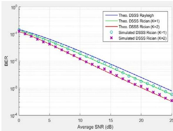
Figure.7 BER performance of non-quantized DSSS with Rician fading channel with K=1, 2
