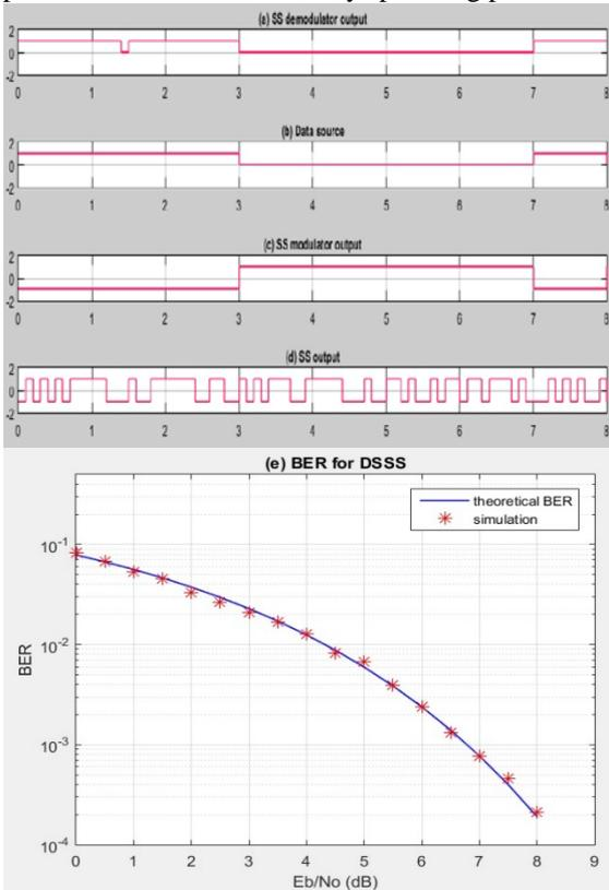
Figure.3 DS signals of 8 seconds Time scope and BER performance for 10 chips/bit DSSS
