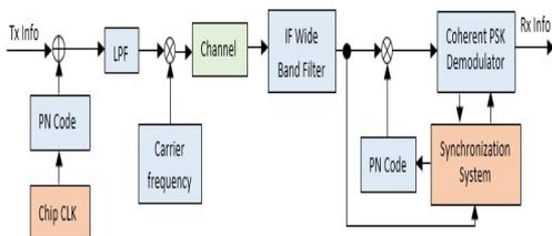
**Figure.1** Model of transmitter and receiver of basic DSSS
