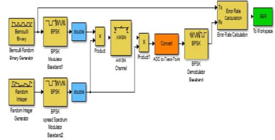
Figure.9 Simulink model of Quantized DSSS with AWGN channel
