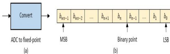
Figure.8 (a) Simulink convert-block, (b) Fixed-point representation
