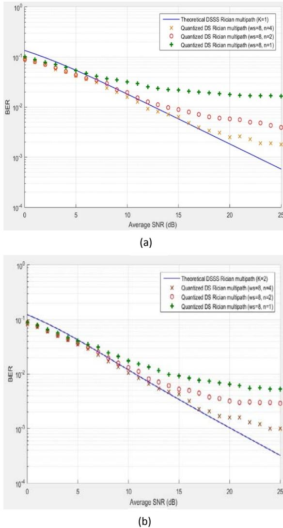
**Figure.16** BER performance of Quantized DSSS with Rician multipath fading channel for different quantization levels ( $n=1, 2,$  and  $4$ ): (a) Rician factor  $K=1,$  (b) Rician factor  $K=2.$
