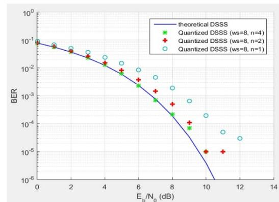
Figure.10 BER performance of Quantized DSSS with AWGN channel
