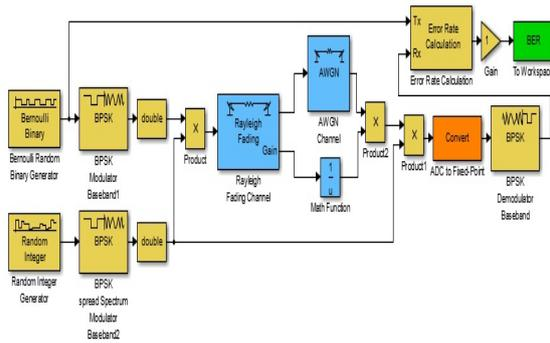
Figure.11 Simulink model of Quantized DSSS affected by Rayleigh fading channel
