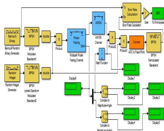
Figure.13 Simulink model of Quantized DSSS affected by multipath Rician fading channel
