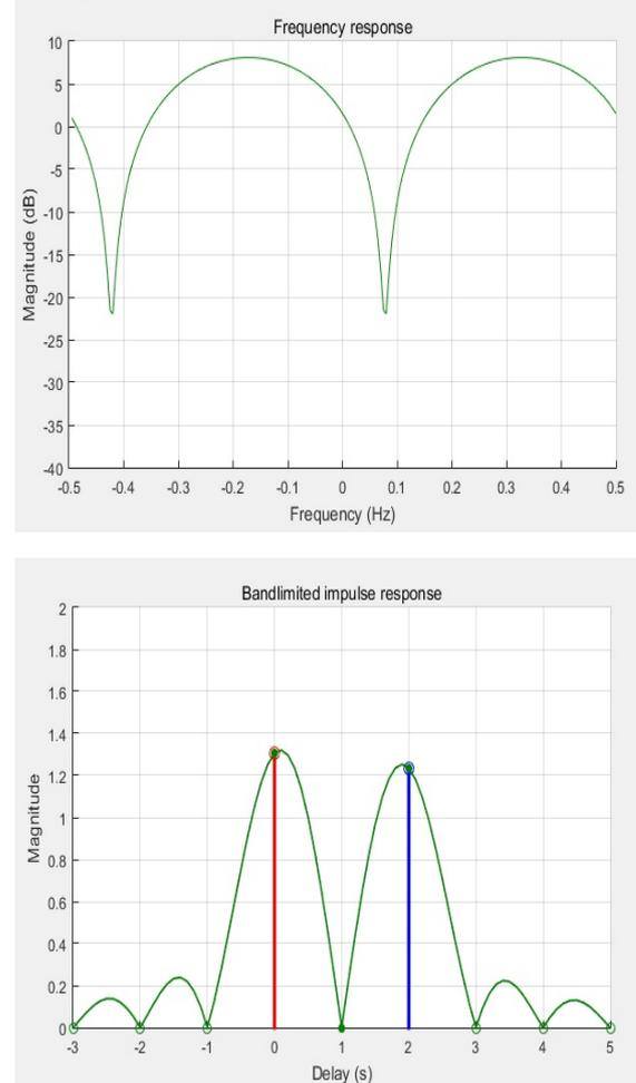
**Figure.15** Frequency response and Impulse response of Rician multipath channel for Rician factor=3 after 10000 samples
