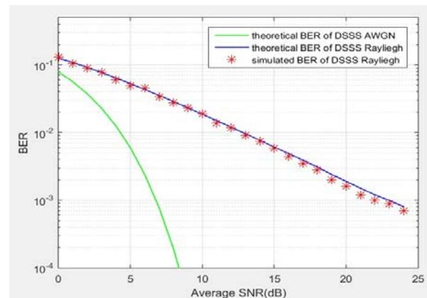
**Figure.6** BER performance of non-quantized DSSS with Rayleigh fading and AWGN channels
