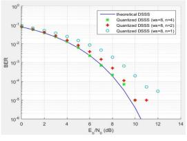
Figure.10 BER performance of Quantized DSSS with AWGN channel
