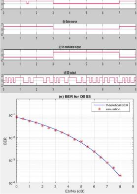
**Figure.3** DS signals of 8 seconds Time scope and BER performance for 10 chips/bit DSSS
