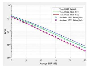
**Figure.7** BER performance of non-quantized DSSS with Rician fading channel with K=1, 2
