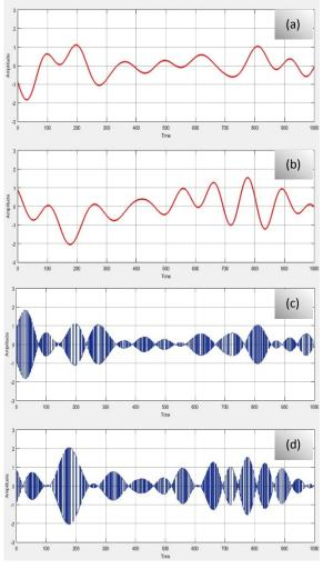
**Figure.5** Real and Imaginary parts of Rayleigh fading channel in Non-quantized DSSS: (a, b) channel Gain, (c, d) channel output
