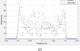
**Figure.14** Rician channel Doppler spectrum for Rician factor=3 and after 10000 samples: (a) Doppler spectrum without multipath, (b) Doppler spectrum for 1<sup>st</sup> path, (c) Doppler
