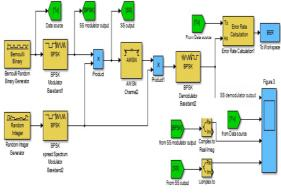
Figure.2 Simulink model of DSSS using BPSK modulation
