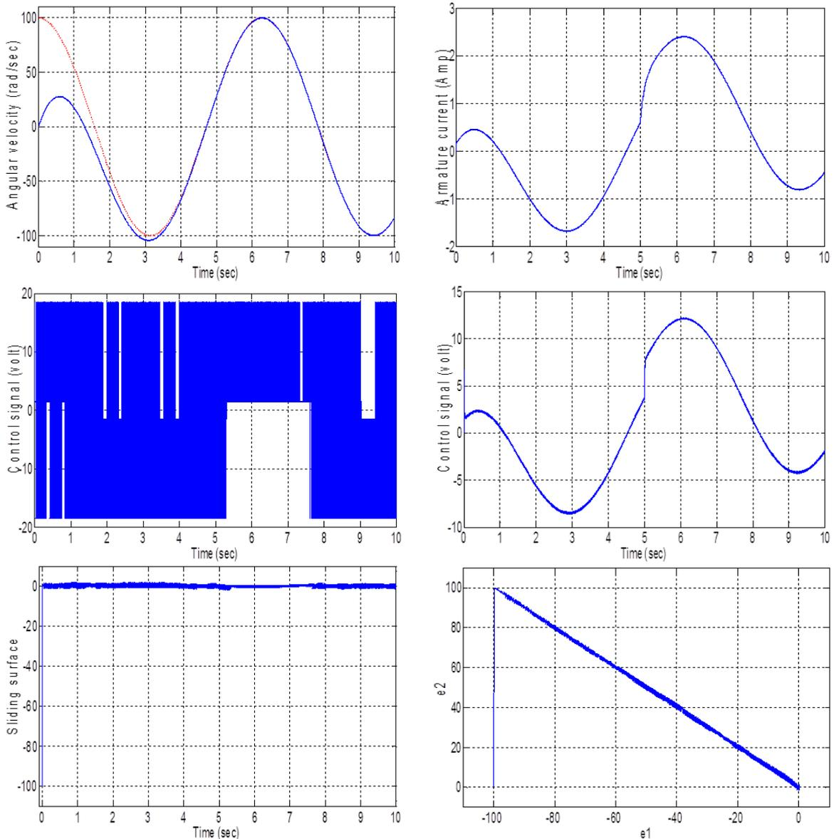
**Figure (4)** Simulation of different system responses due to sinusoidal input with disturbance
