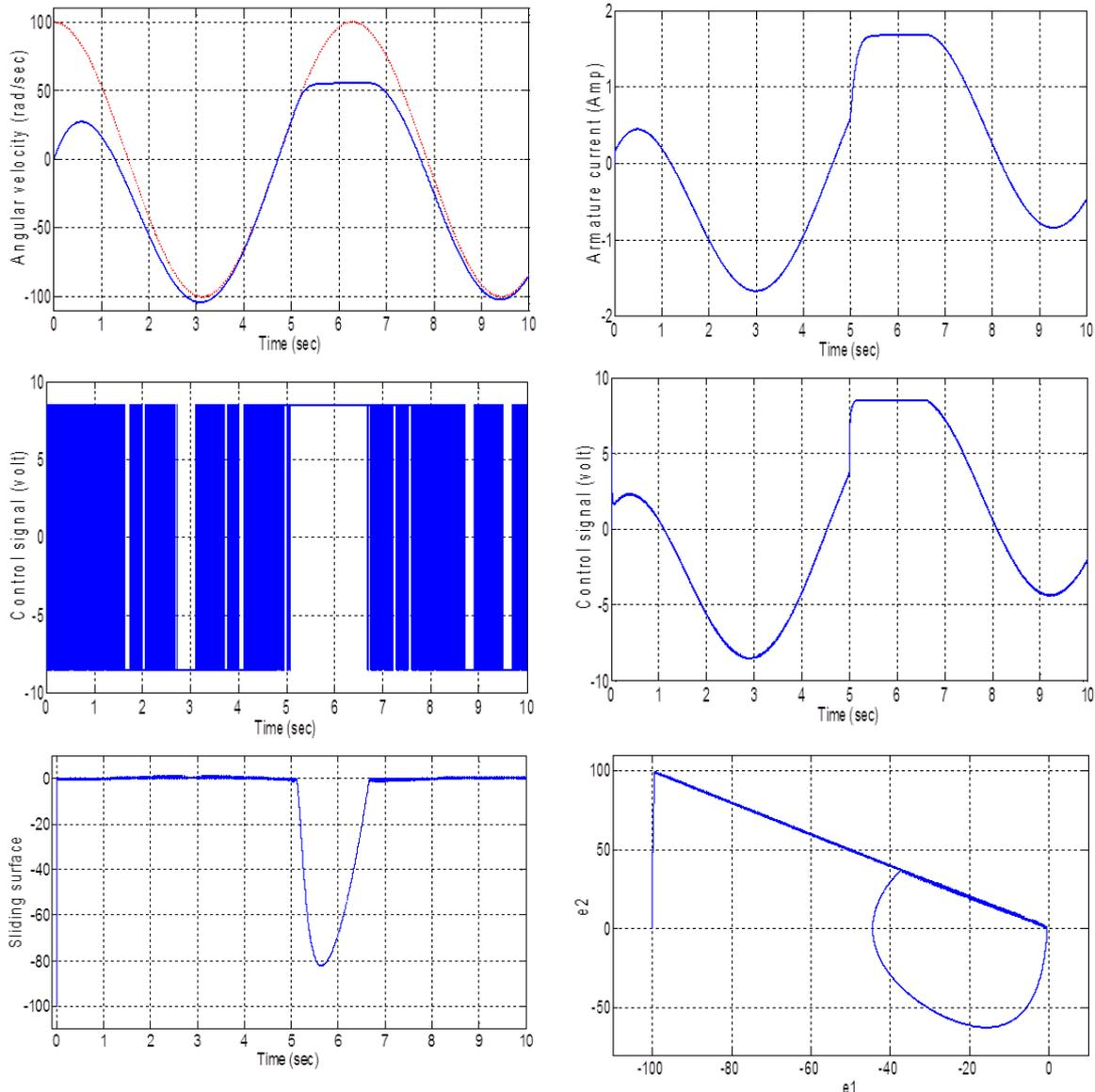
**Figure (3)** Simulation of different system responses due to sinusoidal input without disturbance
