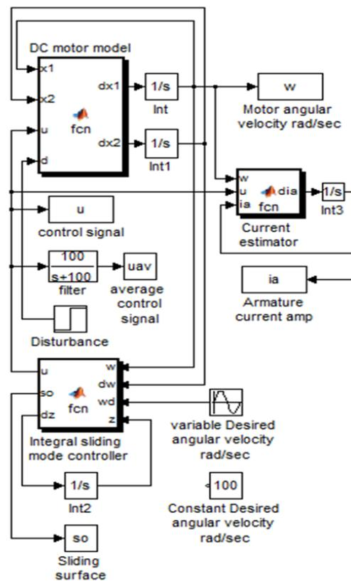
**Figure (1)** Simulink Modeling of Sliding Mode Controller
