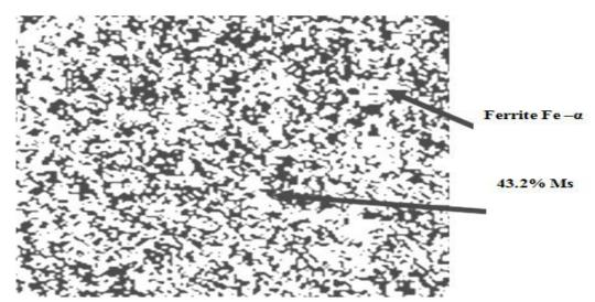
**Figure 6:** The microstructure of the Dual-phase steel ,( $820^{\circ}C$ ) annealing temperature , (X1000) .
