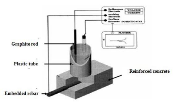
Figure 10: Schematic of the connection between the potentiostat and the three electrodes to the DC corrosion measurement software [11].
