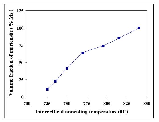
Figure 9: Percentage of volume fraction of martensite vs intercritical annealing temperature ( $^{0}$ C) for the Ukrainian (0.22%C) steel .
