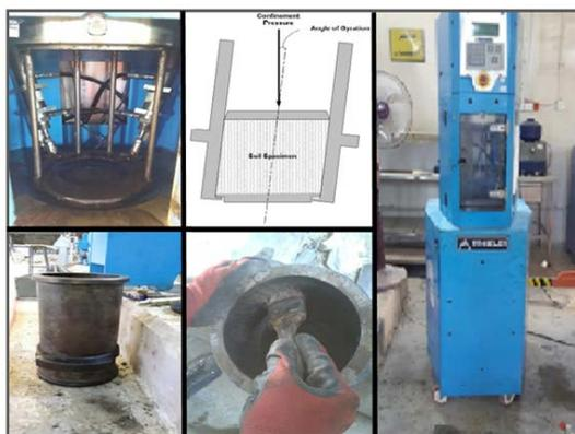
Figure 3: Superpave gyratory compactor, mold and container
