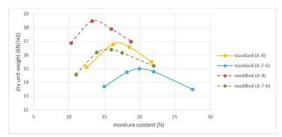
Figure 2: Standard and modified Proctor tests curves
