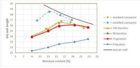
Figure 9: Compaction curves for (A-4) soil under 200 kPa
