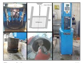
Figure 3: Superpave gyratory compactor, mold and container
