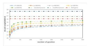
**Figure 5:** UWCC for dry soil type (A-4)
