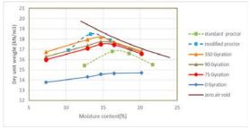
Figure 10: Compaction curves for (A-4) soil under 600 kPa
