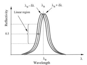
Figure 2: wavelengths Spectrum Shift in the FBG
