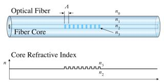
Figure 1: Fiber Bragg Grating structure
