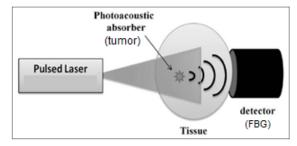
Figure 3: Photoacoustic principle
