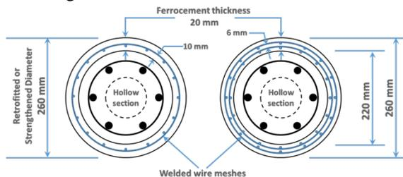
**Figure (4):** Cross section in the ferrocement jacketed column
