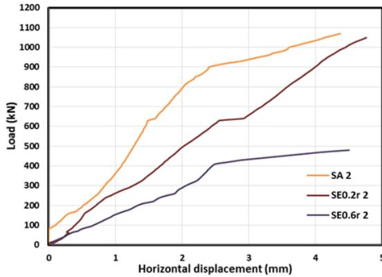
Figure (13): Effect of eccentricity on the (L-HD) curves with two layers of WWM
