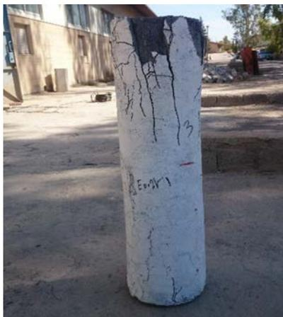
**Figure (17):** Failure mode of RE0.2r 1 column (crushing of concrete and yielding)
