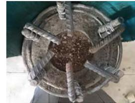
b) Hollow core filling with sand
