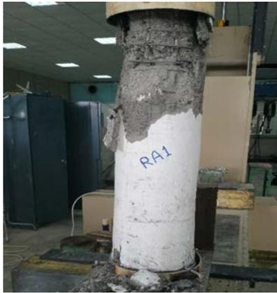
**Figure (16):** Failure mode of RA 1 column (yielding and partially pull off of strengthened layer)
