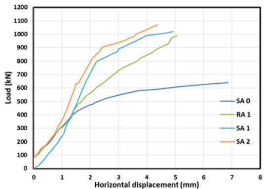
Figure (8): Effect of WWM layers on the (L-HD) curves with  $e = 0$
