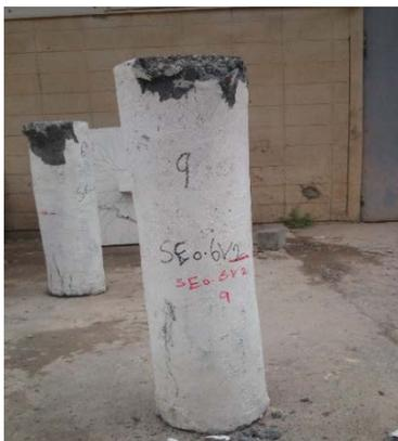
**Figure (23):** Failure mode of SE0.6r 2 column (tension failure with crushing of concrete)
