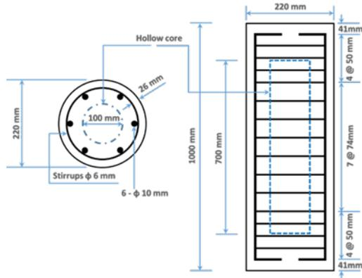
Figure (1): Reinforcement details in the specimen
