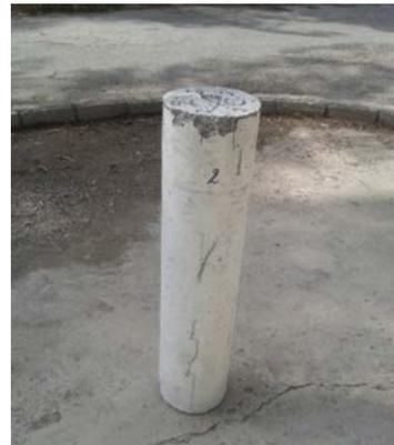
Figure (14): Failure mode of SA 0 column (crushing of concrete)
