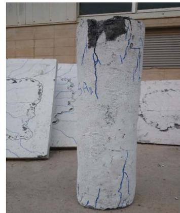
**Figure (21):** Failure mode of SA 2 column (aggressive crushing of concrete)
