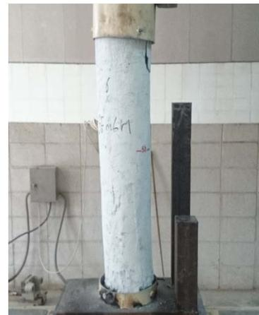
**Figure (20):** Failure mode of SE0.6r 1 column (tension failure)
