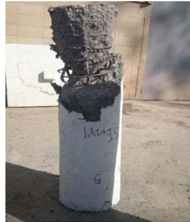
**Figure (19):** Failure mode of SE0.2r 1 column (crushing of concrete with yielding main reinforcement)
