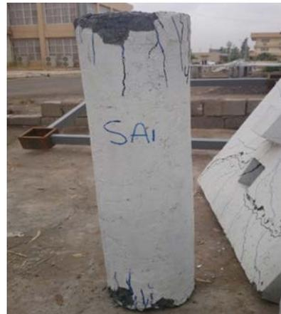
**Figure (18):** Failure mode of SA 1 column (Partially pull off with concrete crushing)
