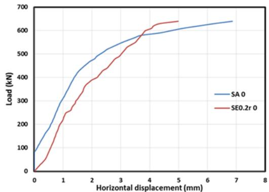
Figure (11): Effect of eccentricity on the (L-HD) curves with zero layer of WWM
