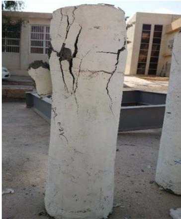
**Figure (22):** Failure mode of SE0.2r 2 column (crushing of concrete with yielding in tension face)
