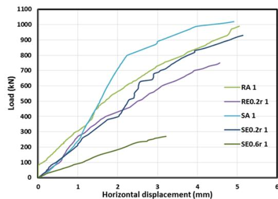
Figure (12): Effect of eccentricity on the (L-HD) curves with one layer of WWM
