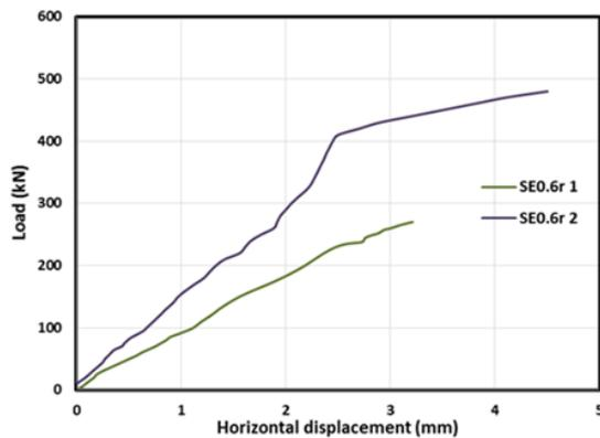
Figure (10): Effect of WWM layers on the (L-HD) curves with  $e = 0.6r$
