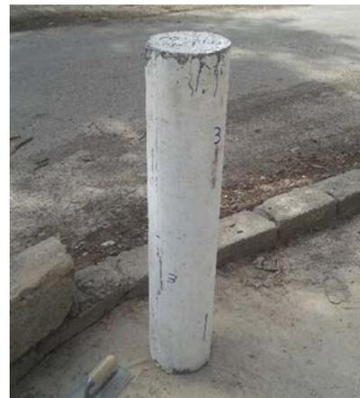
Figure (15): Failure mode of SE0.2r 0 column (crushing of concrete with moderate tension face failure)
