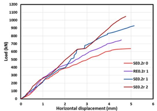
Figure (9): Effect of WWM layers on the (L-HD) curves with  $e = 0.2r$
