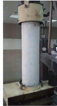
Figure (7): Testing of column specimen
