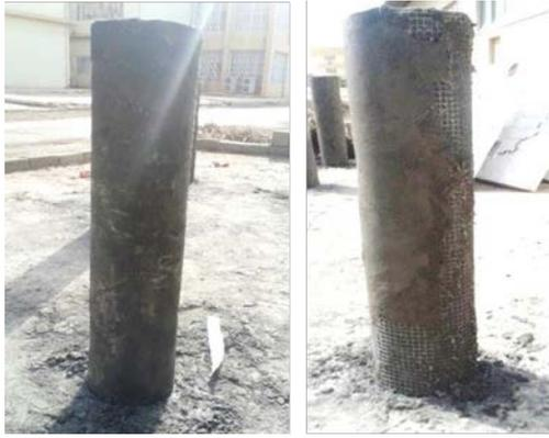
Figure (5): Welded wire mesh wrapping around the column
