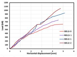
**Figure (9):** Effect of WWM layers on the (L-HD) curves with e = 0.2r
