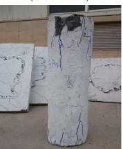
Figure (21): Failure mode of SA 2 column (aggressive crushing of concrete)
