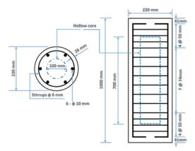
Figure (1): Reinforcement details in the specimen
