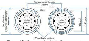
Figure (4): Cross section in the ferrocement jacketed column
