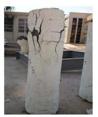
**Figure (22):** Failure mode of SE0.2r 2 column (crushing of concrete with yielding in tension face)
