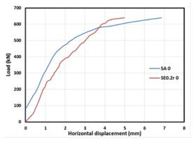
Figure (11): Effect of eccentricity on the (L-HD) curves with zero layer of WWM
