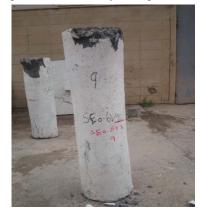
Figure (23): Failure mode of SE0.6r 2 column (tension failure with crushing of concrete)
