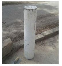
**Figure (15):** Failure mode of SE0.2r 0 column (crushing of concrete with moderate tension face failure)
