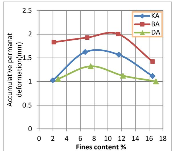
Figure (9) Fines content – accumulative permanent deformation relationship (unsoaked samples)
