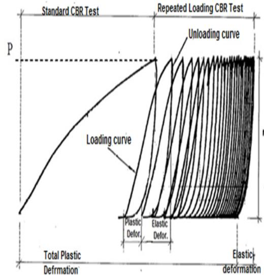
Figure 4: Repeated load CBR test principle (Molenaar, 2008)
