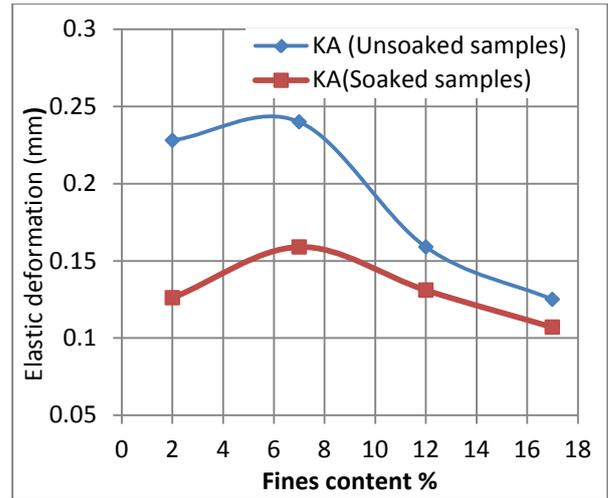
Figure (6) Fines content – Elastic deformation relationship for material (KA)
