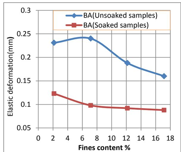
Figure (7) Fines content – Elastic deformation relationship for material (BA)
