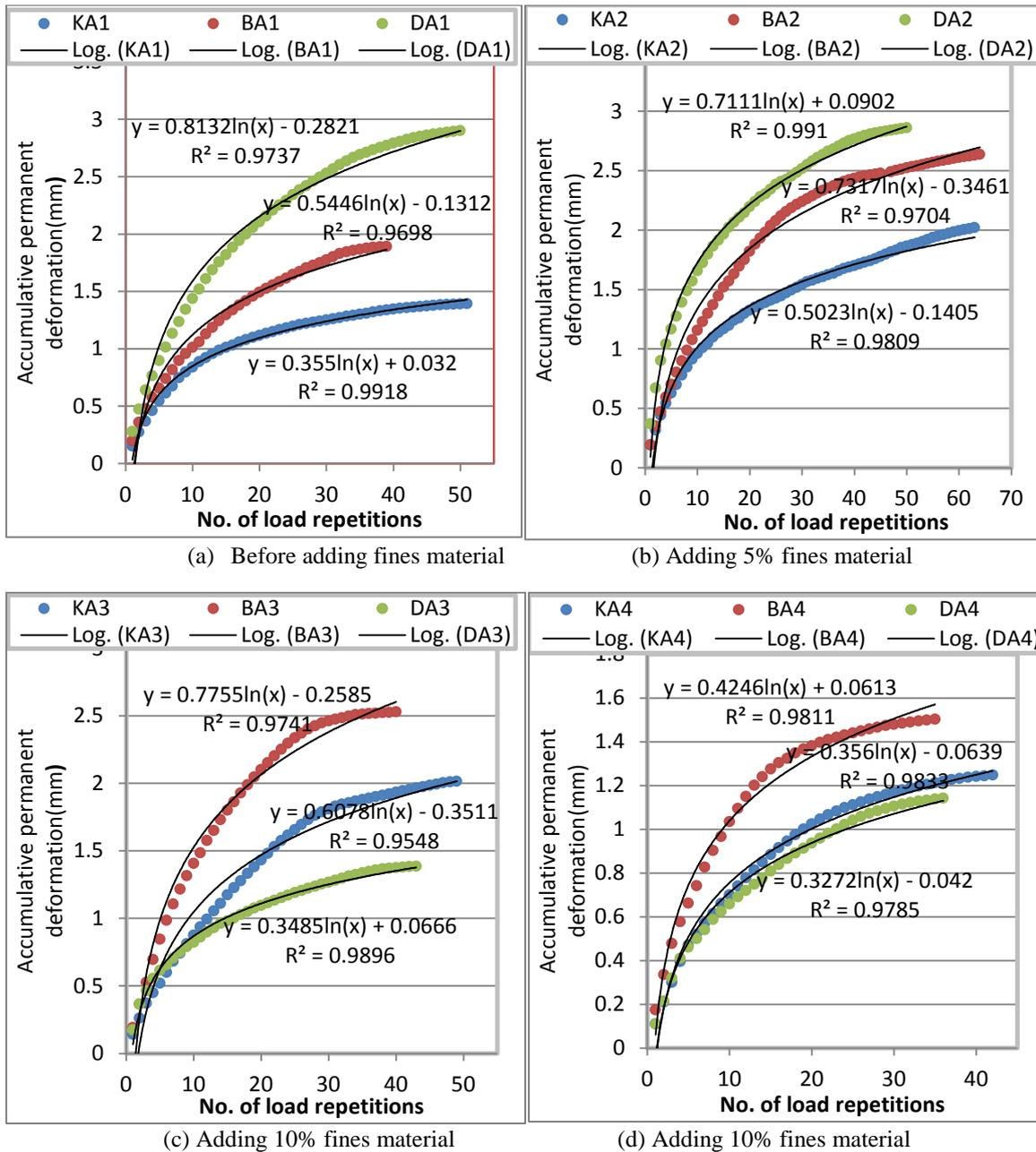
Figure 14: Correlation of accumulative deformation with number of load repetitions (soaked samples)
