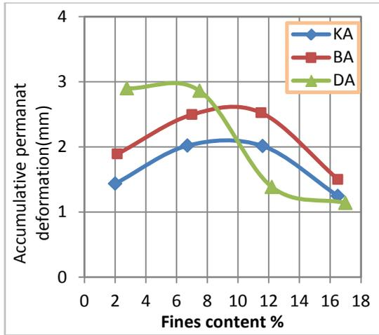
Figure (10) Fines content – accumulative permanent deformation relation (soaked samples)
