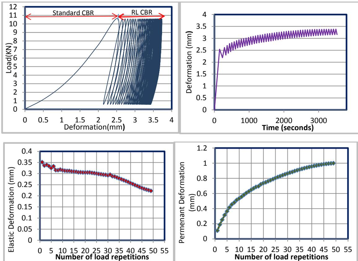
Figure 5: Repeated load CBR test
