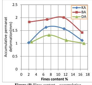
**Figure (9)** Fines content – accumulative permanent deformation relationship (unsoaked samples)
