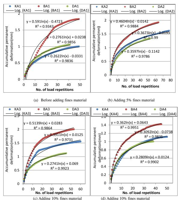
(c) Adding 10% fines material (d) Adding 10% fines material **Figure 13:** Correlation of accumulative deformation with number of load repetitions (unsoaked samples)
