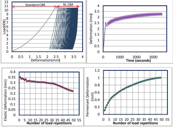
Figure 5: Repeated load CBR test
