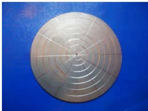
Figure (6): the sheet with grids, by using mechanical grid marker
