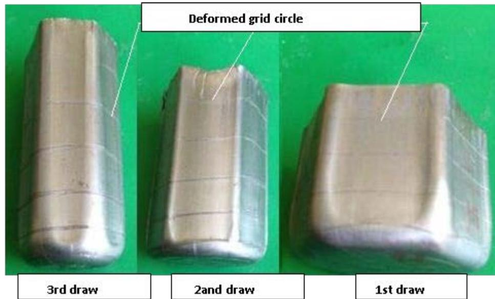
Figure (7): the distortion of grid on hexagonal cup in three stages.
