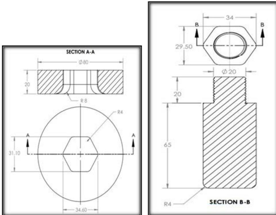
Figure (4): The die and punch in second step schematically
