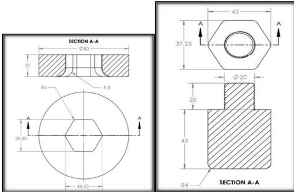
Figure (3): The die and punch in first step schematically
