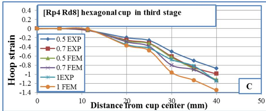
Figure (14): Influence of sheet thickness on hoop strain in three stages
