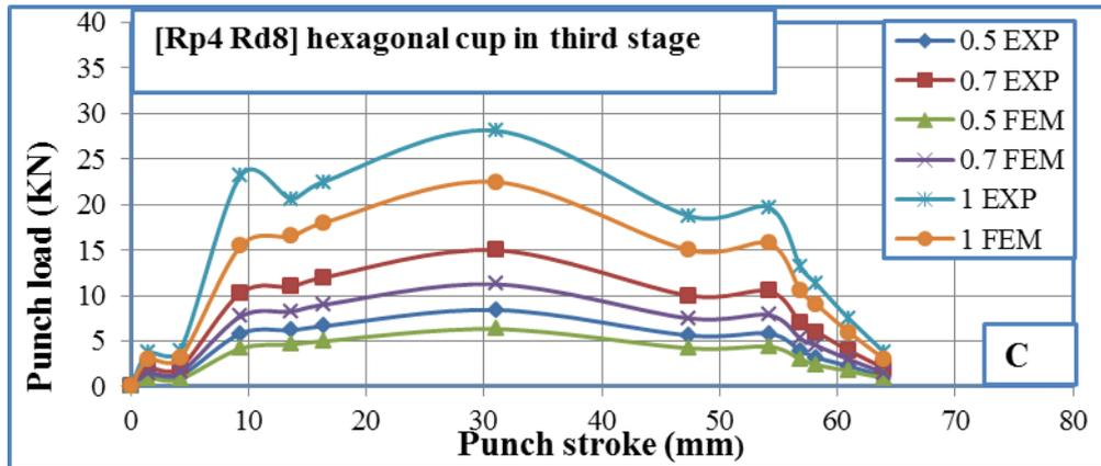
Figure (10): influence of sheet thickness on punch force in three stages
