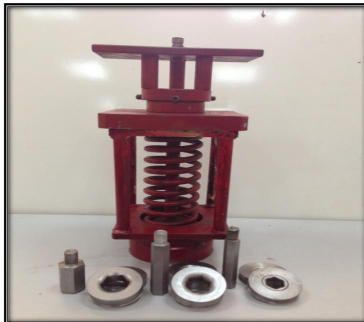
Figure (2): The picture of deep drawing tools used
