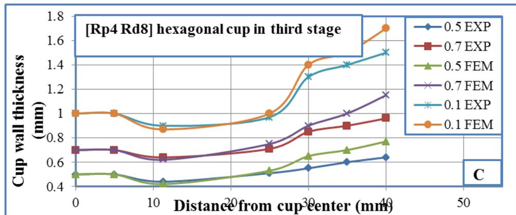
Figure (11): Influence of sheet thickness on cup wall thickness in three stages
