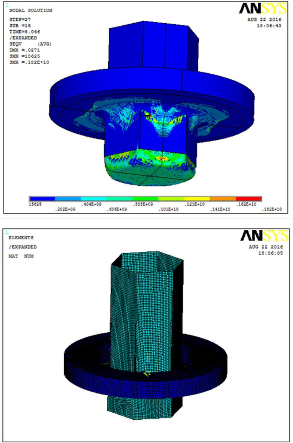
Figure (8): Finite element model of the sheet material and forming Hexagonal
