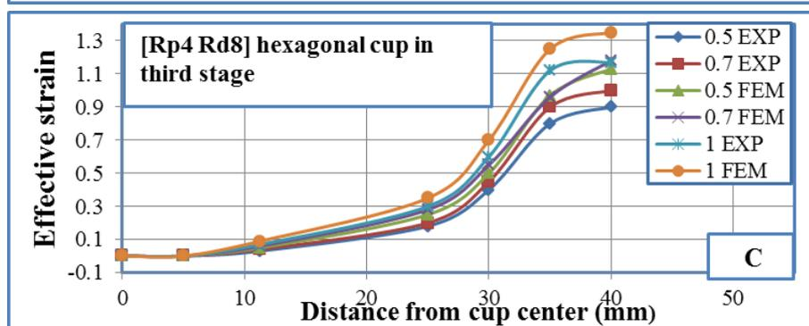
Figure (15): Influence of sheet thickness on effective strain in three stages
