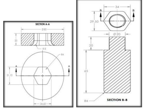
Figure (4): The die and punch in second step schematically
