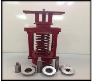
Figure (2): The picture of deep drawing tools used
