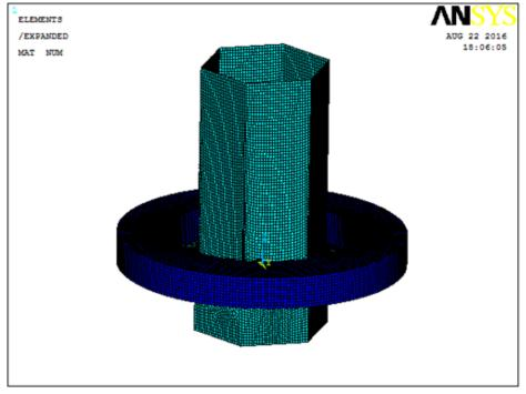
Figure (8): Finite element model of the sheet material and forming Hexagonal
