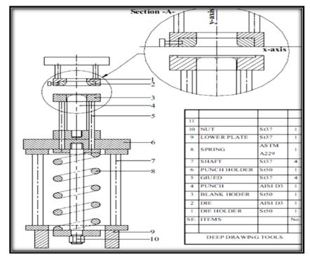
Figure (1): The schematic of deep drawing tools used
