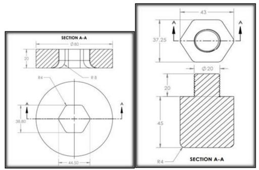
Figure (3): The die and punch in first step schematically
