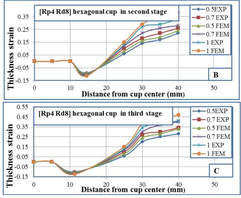
Figure (13): influence of sheet thickness on thickness strain in three stages
