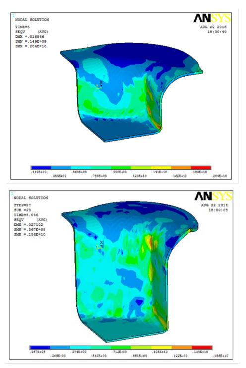
Figure (9): A successive final stage of the deep forming sheet
