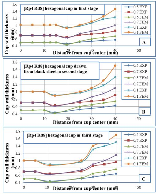
Figure (11): Influence of sheet thickness on cup wall thickness in three stages
