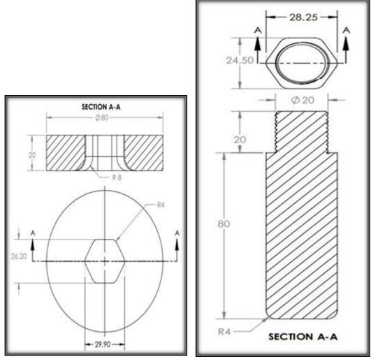
Figure (5): The die and punch in third step schematically
