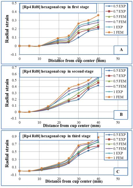
Figure (12): Influence of sheet thickness on radial strain in three stages
