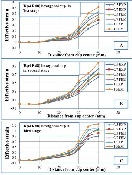
Figure (15): Influence of sheet thickness on effective strain in three stages
