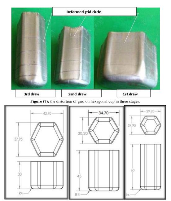
Figure (8): The cup for three steps schematically
