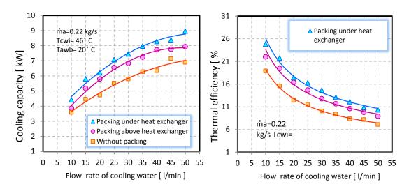
Figure 21: Variation of cooling capacity with cooling water flow rate for different locations of packing
