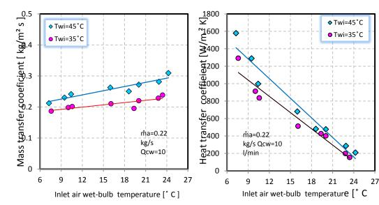
**Figure 17:** Variation of mass transfer coefficient with inlet AWBT for different inlet water temperatures
