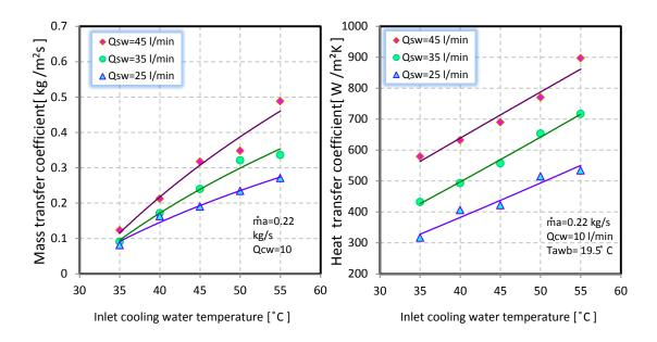
Figure 13: Variation of mass transfer coefficient with inlet cooling water temperature for different inlet water temperatures
