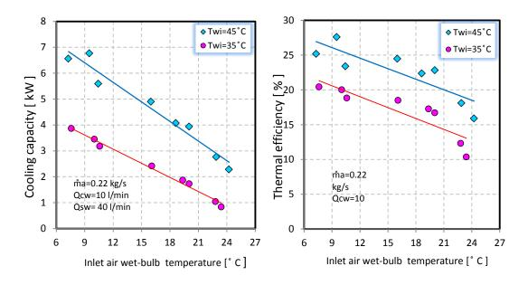
Figure 15: Variation of cooling capacity with inlet AWBT for different inlet water
