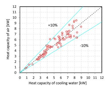
Figure 2: Energy balance of the experimental apparatus
