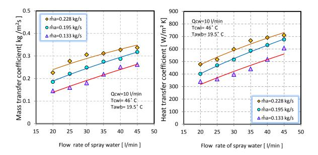
**Figure 5:** Variation of mass transfer coefficient with spray water flow rate for different air flow rates
