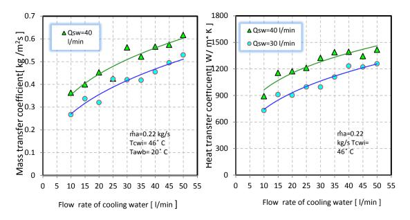
**Figure 9:** Variation of mass transfer coefficient with cooling water flow rate for different spray water flow rates
