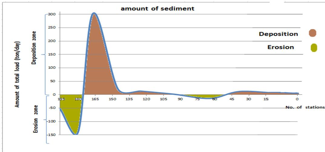
Figure (8): Total load results for main cross-sections, (erosion or deposition)
