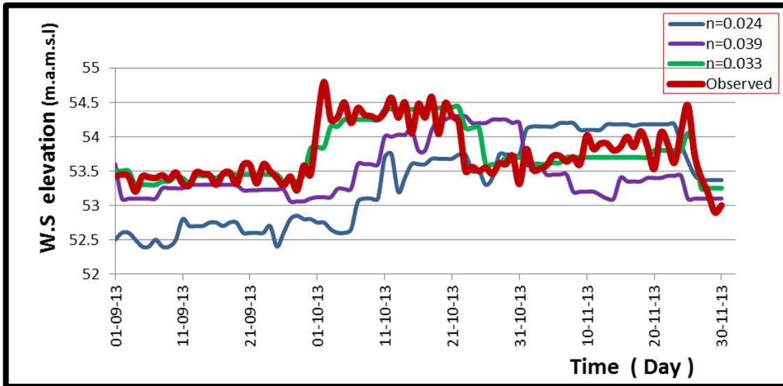
Figure (7): Calculated and Observed Water Surface Elevation at Heet Station for different values of Manning's (n)
